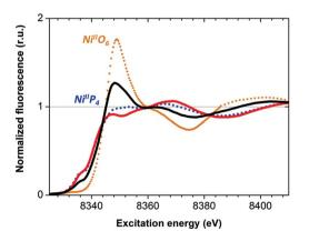
Fig. 4 X-ray absorption near edge structure spectra (Ni K edge) of the Ni-CNT material as prepared (black solid line), and after 1 h H<sub>2</sub> oxidation (red solid line). Spectra of pristine [Ni(P<sub>2</sub><sup>Ph</sup>N<sub>2</sub><sup>CH<sub>2</sub>pyrene</sup>)<sub>2</sub>] (blue dotted line) and of [Ni(OH<sub>2</sub>)<sub>6</sub>]<sup>2+</sup> (orange dotted line) are shown for comparison. See Fig. S10† for a magnification of the K edge region.
