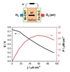
Fig. 2 Left: schematic description of the PEMFC assembly; right: polarization and power density curves of the Ni–CNT/Co–N–C PEMFC recorded at 60  $^{\circ}$ C with a supply of partially humidified H<sub>2</sub> (20 mL min $^{-1}$ ) at the anode and passive air convection at the cathode.
