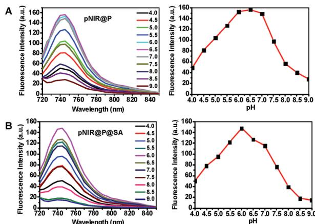
Fig. 3 pH correlated fluorescence of pNIR@P (A) and pNIR@P@SA (B). The two polymersomes were spiked into sodium phosphate buffer (100 mM, pH 4.0–9.0) to a final concentration of  $100 \mu\text{g ml}^{-1}$ . Fluorescence emission of the solutions was recorded using  $\lambda_{\text{ex}}@715 \text{ nm}$  and fluorescence emission intensities@745 nm were plotted over buffer pH.
