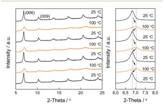
Fig. 7 The reversible change in the XRD pattern of CoAl–AO5 upon heating and cooling. The magnified XRD pattern (right) highlights the movement and broadness increase of the (006) peak.
