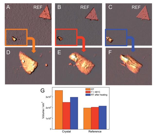
Fig. 9 AFM images of CoAl-AO5 acquired at ambient conditions and different temperatures. In each image we can distinguish a crystal and a reference marker: (A) RT; (B) 80 °C; (C) RT after heating the sample at 80 °C. Image size: 17 μm × 17 μm. (D), (E) and (F) correspond to magnifications of (A), (B), (C) respectively to observe in detail the evolution of the shape of the crystal. (G) Histogram of the volume of CoAl-AO5 and the reference measured by AFM.
