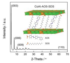
Fig. 4 X-ray diffraction pattern of CoAl-AO5.
