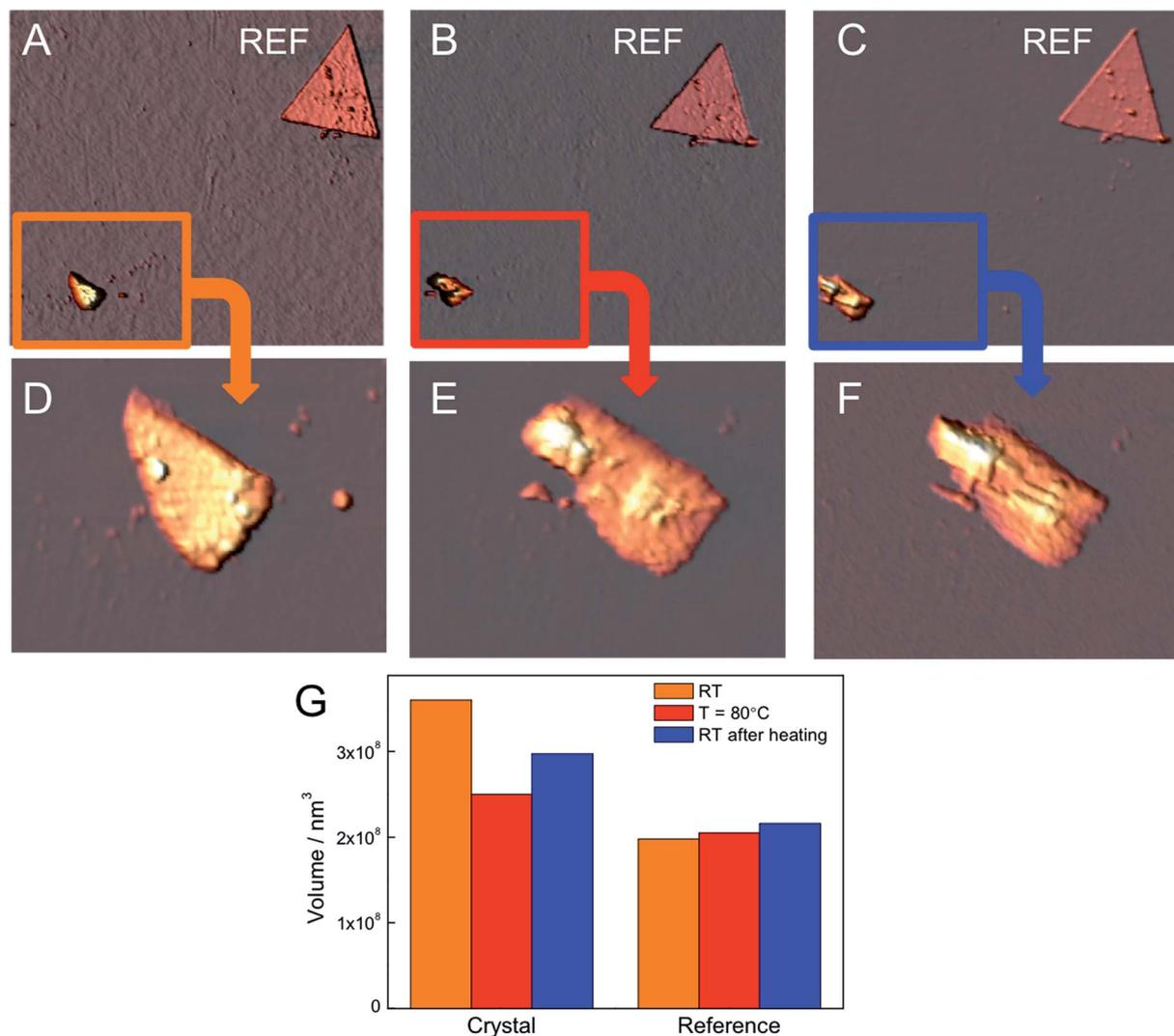
Fig. 9 AFM images of CoAl-AO5 acquired at ambient conditions and different temperatures. In each image we can distinguish a crystal and a reference marker: (A) RT; (B) 80 °C; (C) RT after heating the sample at 80 °C. Image size: 17  $\mu\text{m}$   $\times$  17  $\mu\text{m}$ . (D), (E) and (F) correspond to magnifications of (A), (B), (C) respectively to observe in detail the evolution of the shape of the crystal. (G) Histogram of the volume of CoAl-AO5 and the reference measured by AFM.
