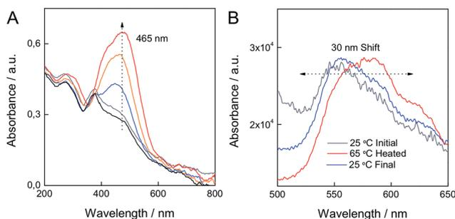
Fig. 6 (A) *In situ* transmission absorption spectra of the CoAl-AO5 film during heating in the temperature range 25–80 °C. (B) The corresponding *in situ* fluorescence spectra showing the reversible peak shift after heating at 65 °C.
