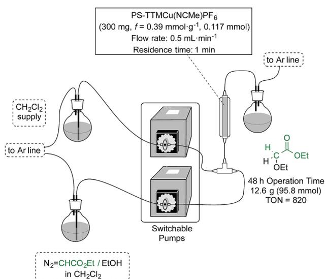
Fig. 1 The experimental setup for continuous flow operation.
