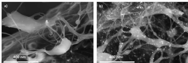
Fig. 2 High resolution SEM images of (a) as received and (b) 46 wt% Pt-decorated commercial CNTs. Pt nanoparticles with diameters of <17 nm are evident in the latter. Bundling and agglomeration of CNTs is evident in both images.
