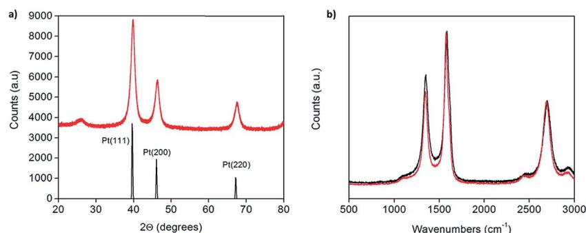
Fig. 1 (a) X-ray powder diffraction of 46 wt% Pt-CNTs (red) along with a reference trace<sup>25</sup> (black), and (b) Raman spectra of as-received (red) and 46 wt% Pt-decorated (black) commercial CNTs showing that the carbon nanotube structure is largely unchanged after decoration.
