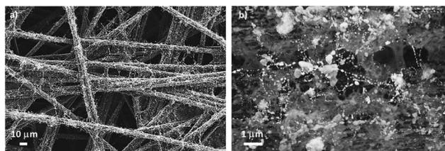
Fig. 5 SEM images of electrospayed 46 wt% Pt-CNT–CsH<sub>2</sub>PO<sub>4</sub> composites, showing direct contact between the electrolyte particles with the carbon nanotubes: (a) low and (b) high magnification.
