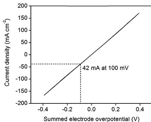
Fig. 8 IR-corrected polarization curve of a 46 wt% Pt-CNT-CsH<sub>2</sub>PO<sub>4</sub> composite electrode at 1 mV s<sup>-1</sup>, showing high current density at low overpotentials for both proton reduction and hydrogen oxidation.
