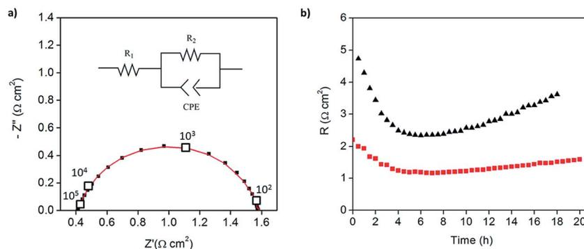
Fig. 7 Symmetric cell impedance measurements Pt-CNT based electrodes prepared by strategy 2: (a) Nyquist plot for 46 wt% Pt-CNT-CsH<sub>2</sub>PO<sub>4</sub> composite after 4 hours (inset: equivalent circuit used for fitting) and (b) temporal evolution of the electrode resistance values of 30 wt% (black) and 46 wt% (red) Pt-CNT-CsH<sub>2</sub>PO<sub>4</sub> composites, showing higher stability in the electrolyte with higher Pt loading.
