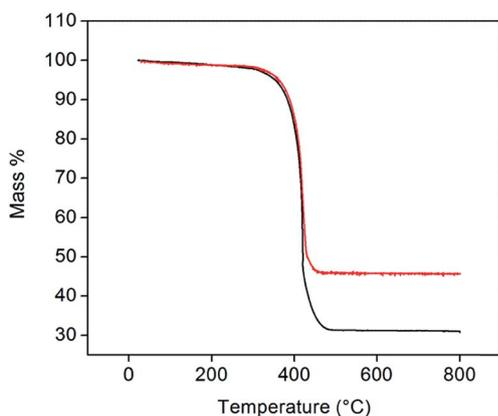
Fig. 3 TGA profiles of 30 (black) and 46 wt% (red) Pt-CNTs (measured under flowing air at a heating rate of 2 °C min<sup>-1</sup>).
