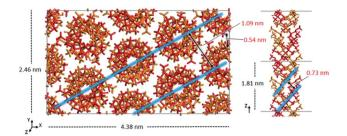
Fig. 4 Model of the optimized crystal structure of  $9_1$  it-PMMA in the Right Down packing motif. The chain-chain spacing (left) and pitch spacing (right) are shown in light blue.
