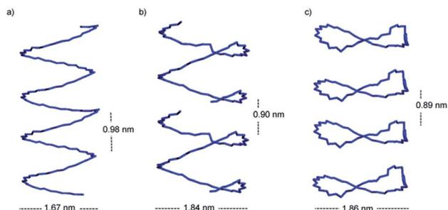
Fig. 7 The syndiotactic helix backbone of the (a)  $9_1$ -it/18 $_1$ -st (b)  $9_1$ -it/40mer-st and (c)  $9_1$ -it/cyclic-18mer-st stereocomplex models. The it-PMMA double helix is not shown. The larger diameter of the  $9_1$ -it/40mer-st and distinct helical curvature of this model enable the fit to the experimental X-ray diffraction peaks at 2.08 nm and 0.78 nm, respectively.
