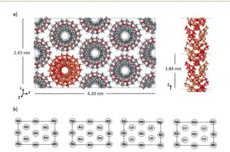
Fig. 1 a) Initial model crystal structure of  $9_1$  it-PMMA, (b) the four packing motifs examined in this study (from left to right): Right Down (RD), Right Down/Right Up (RD/RU), Right Down/Left Down (RD/LD), and Right Down/Left Up (RD/LU).
