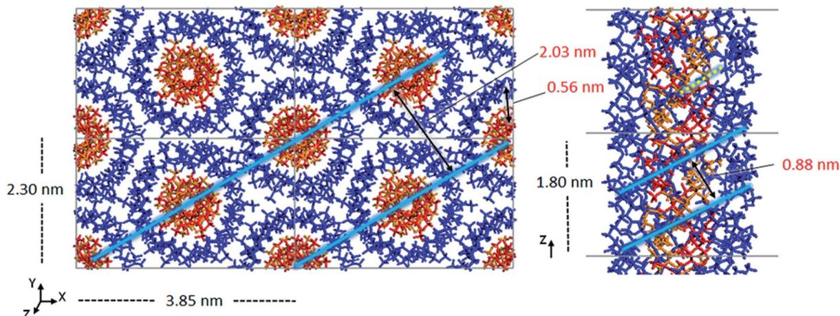
**Fig. 6** Optimized crystal structure model of 9<sub>1</sub>-it-/40mer-st-PMMA in the Right Down packing motif. The chain–chain spacing (left) and pitch spacing (right) are shown in light blue. The gap between 40-unit st-PMMA fragments is shown by a dotted yellow line.
