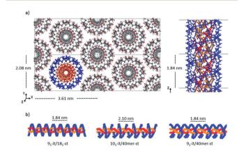
Fig. 2 a) Initial model crystal structure of the  $9_1$ -it-/ $18_1$ -st-PMMA stereocomplex, (b) schematic representations of the three triple helix stereocomplex systems.
