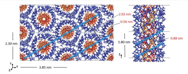
Fig. 6 Optimized crystal structure model of 91-it-/40mer-st-PMMA in the Right Down packing motif. The chain-chain spacing (left) and pitch spacing (right) are shown in light blue. The gap between 40-unit st-PMMA fragments is shown by a dotted yellow line.
