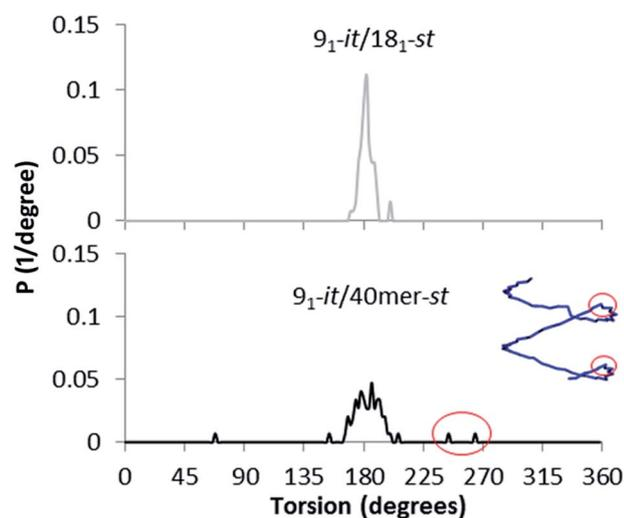
Fig. 8 Backbone torsion distribution of the st-PMMA in the it-/st-PMMA stereocomplex models. The  $9_1$ -it/18 $_1$ -st model represents an ideal helix, while the  $9_1$ -it/40mer-st model exhibits non-ideal helical geometry. The torsions associated with this non-ideal helical geometry are circled in red.
