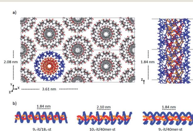
Fig. 2 a) Initial model crystal structure of the 9<sub>1</sub>-it-/18<sub>1</sub>-st-PMMA stereocomplex, (b) schematic representations of the three triple helix stereocomplex systems.
