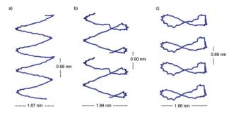
Fig. 7 The syndiotactic helix backbone of the (a)  $9_1$ -it/ $18_1$ -st (b)  $9_1$ -it/ 40mer-st and (c) 9<sub>1</sub>-it/cyclic-18mer-st stereocomplex models. The it-PMMA double helix is not shown. The larger diameter of the 9<sub>1</sub>-it/ 40mer-st and distinct helical curvature of this model enable the fit to the experimental X-ray diffraction peaks at 2.08 nm and 0.78 nm, respectively.
