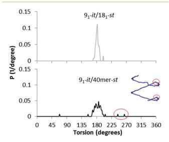
Fig. 8 Backbone torsion distribution of the st-PMMA in the it-/st-PMMA stereocomplex models. The 9<sub>1</sub>-it/18<sub>1</sub>-st model represents an ideal helix, while the 9<sub>1</sub>-it/40mer-st model exhibits non-ideal helical geometry. The torsions associated with this non-ideal helical geometry are circled in red.
