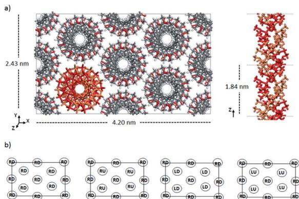
Fig. 1 a) Initial model crystal structure of 9<sub>1</sub> it-PMMA, (b) the four packing motifs examined in this study (from left to right): Right Down (RD), Right Down/Right Up (RD/RU), Right Down/Left Down (RD/LD), and Right Down/Left Up (RD/LU).
