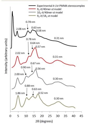
Fig. 5 Wide angle X-ray scattering data obtained from powder diffraction experiments and molecular dynamic simulation for the it-/st-PMMA stereocomplex in the Right Down packing motif.
