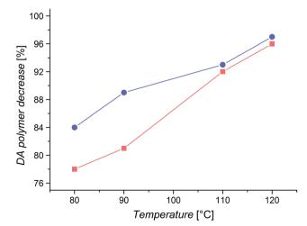
Fig. 12 TD SEC results: decrease of concentration of DA polymer due to rDA reaction of the DA polymers consisting of Cp difunctional  $PMA_{large}$  ( $\blacksquare$ , 50 repeating units) and  $P^{i}BoA_{large}$  ( $\blacksquare$ , 50 repeating units) building blocks and CDTE dilinker.
