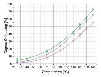
Fig. 8 Temperature dependent degree of debonding for Diels-Alder polymers consisting of Cp difunctional  $P^{i}BuA$  ( $\blacktriangleright$ ),  $P^{n}BuA$  ( $\spadesuit$ ) or  $P^{t}BuA$ (★) building blocks with a length of 50 repeating units and CDTE dilinker assessed by HT NMR spectroscopy
