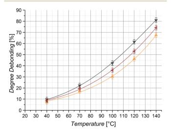
Fig. 6 Temperature dependent degree of debonding for Diels-Alder A,A'-type diblockcopolymers consisting of PMMA ( $\blacktriangle$ ), P'BuMA ( $\blacktriangledown$ ) or PtBuMA ( $\blacktriangleleft$ ) building blocks with a length of 50 repeating units assessed by HT NMR spectroscopy.
