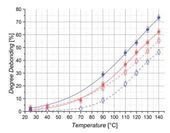
Fig. 11 Temperature dependent degree of debonding for Diels-Alder polymers consisting of Cp difunctional PMA<sub>large</sub> (■, 50 repeating units), P<sup>i</sup>BoA<sub>large</sub> (●, 50 repeating units), PMA<sub>small</sub> (□, 10 repeating units) or PiBoA<sub>small</sub> (O, 10 repeating units) building blocks and CDTE dilinker assessed by HT NMR spectroscopy
