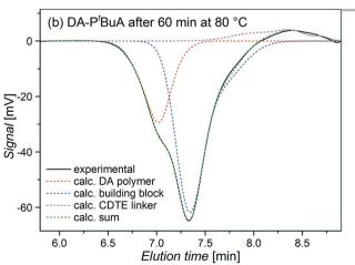
Fig. 9 TD SEC chromatograms, (a) DA-P<sup>t</sup>BuA after different rDA times at 80 °C in 60% TCB and 40% DMF, (b) DA-P<sup>t</sup>BuA after 60 min. rDA at 80 °C and distributions calculated by peak deconvolution of the individual components.
