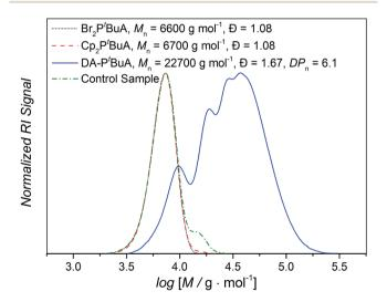
Fig. 7 Exemplary SEC chromatograms of the dibromo precursor polymer (···), Cp difunctional macromonomer (--), Diels-Alder polymer (-) and control sample of heated Cp difunctional macromonomer without CDTE dilinker (---) for 50 tert-butyl acrylate repeating units (see Fig. S2† for the chromatograms of the other employed polymers).
