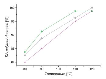
Fig. 10 TD SEC results: decrease of concentration of DA polymers due to rDA reactions of the DA polymers consisting of Cp difunctional  $P^{I}BuA$  ( $\blacktriangleright$ ),  $P^{n}BuA$  ( $\spadesuit$ ) or  $P^{t}BuA$  ( $\bigstar$ ) building blocks with a length of 50 repeating units and CDTE dilinker.
