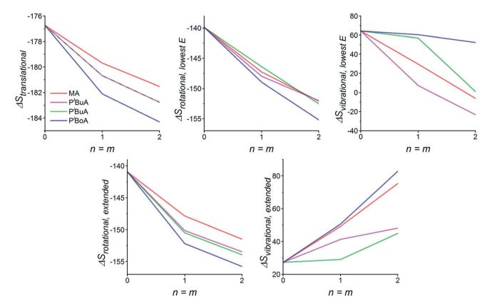
Fig. 3 Calculated changes in the entropy ( $\Delta S$  in J mol<sup>-1</sup> K<sup>-1</sup>) of model DA reactions for different n, m (chain lengths) of various acrylate macromonomers in their lowest energy or extended chain conformation. In these figures, the more negative  $\Delta S$ , the lower the Gibbs free energy of bonding, or the greater the extent of debonding, at a given temperature.
