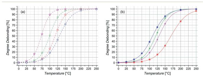
Fig. 4 Degree of debonding (determined from the calculated reaction energies for n = m = 2 chain lengths) vs. temperature for (a) lowest energy and (b) extended chain conformers of P<sup>t</sup>BuA (★), P<sup>i</sup>BuA (▶), PMA (■) or P<sup>i</sup>BoA (●).
