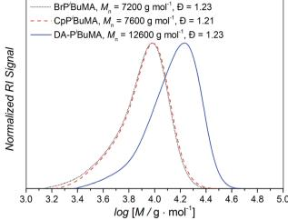
Fig. 5 Exemplary SEC chromatograms of the bromo precursor polymer  $(\cdots)$ , Cp functional building block (--) and Diels-Alder diblock polymer (-) for 50 iso-butyl methacrylate repeating units per building block (see Fig. S1† for the chromatograms of the other employed polymers).
