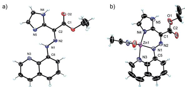
Fig. 2 ORTEP drawings (50% probability ellipsoids) of (a) **1(E)** and (b) **1(Zn-E)**. The protons are placed in calculated positions, except for those of the hydrazone N(1) atom, the imidazolyl nitrogen atoms N(4)/N(5), and the water molecule, which were refined. The counter ion of **1(Zn-E)** is not shown for clarity.
