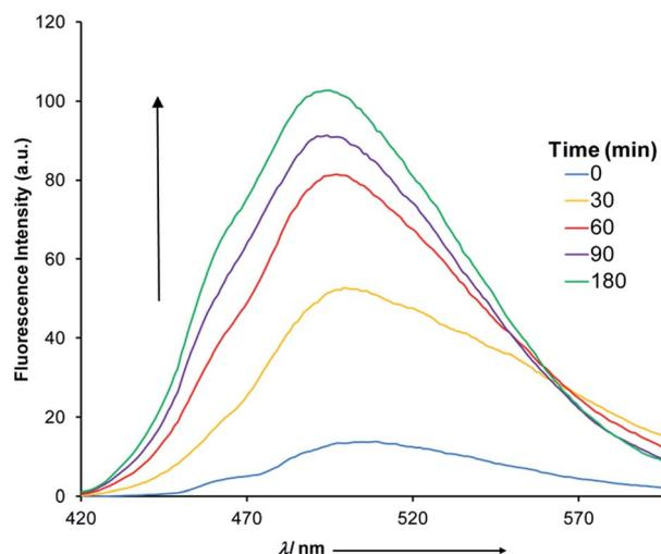
Fig. 5 The fluorescence spectra ( $5 \times 10^{-5}$  M, CH<sub>3</sub>CN) obtained through the CCD mediated catalytic hydrolysis of **ANI**.
