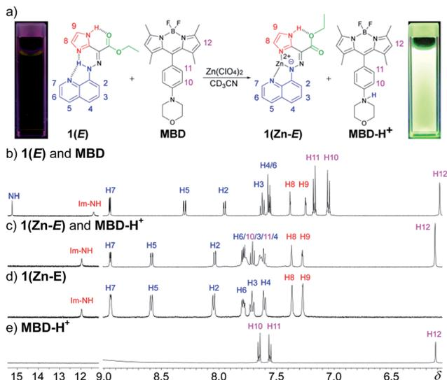
Fig. 1 (a) The compounds involved in the CCD initiated signaling event that turns "on" the emission of MBD. The  $^1\text{H}$  NMR spectra (500 MHz,  $\text{CD}_3\text{CN}$ ) of (b) **1(E)** and **MBD** (1 : 1 mixture); (c) **1(Zn-E)** and **MBD-H<sup>+</sup>** obtained after the addition of 1 equiv. of zinc(II); (d) dissolved crystals of **1(Zn-E)**; and (e) **MBD-H<sup>+</sup>** obtained after addition of TFA (8 equiv.) to **MBD**.
