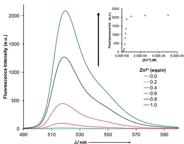
Fig. 3 Fluorescence spectra ( $5 \times 10^{-5} \text{ M}$ ,  $\text{CH}_3\text{CN}$ ) of a 1 : 1 mixture of **1(E)** and **MBD** as a function of zinc(II) equivalents. The inset shows the 1000-fold increase in emission intensity.
