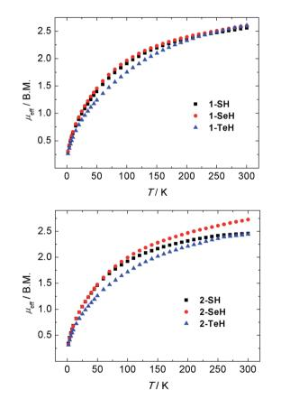
Fig. 4 Temperature-dependent SQUID magnetization data of hydrochalcogenido complexes 1-EH (top, E = S (black), Se (red), Te (blue)) and 2-EH (bottom, E = S (black), Se (red), Te (blue)) as a plot of  $\mu_{\rm eff}$  vs. T. Data were corrected for underlying magnetism.
