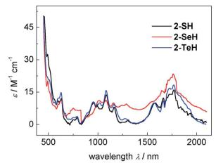
Fig. 3 Vis/NIR spectra of hydrochalcogenido complexes 1-SH (9.2 mM, black), 1-SeH (9.7 mM, red), and 1-TeH (4.1 mM, blue) recorded in DME at 25 °C (left) and vis/NIR spectra of hydrochalcogenido complexes 2-SH (2.0 mM, black), 2-SeH (6.6 mM, red), and 2-TeH (6.5 mM, blue) recorded in benzene at 25 °C (right). The molar extinction coefficients for complexes 2-EH were calculated per uranium center for a better comparison.
