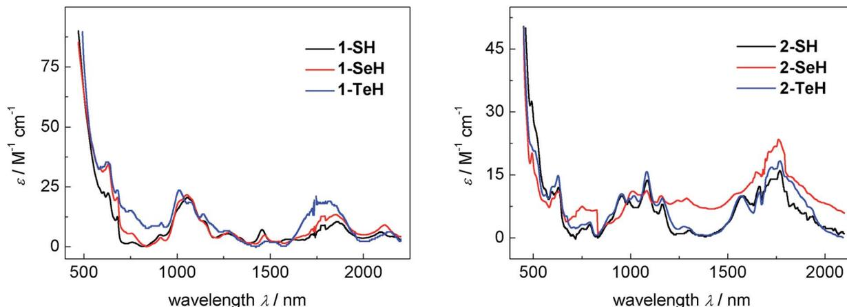
Fig. 3 Vis/NIR spectra of hydrochalcogenido complexes **1-SH** (9.2 mM, black), **1-SeH** (9.7 mM, red), and **1-TeH** (4.1 mM, blue) recorded in DME at 25 °C (left) and vis/NIR spectra of hydrochalcogenido complexes **2-SH** (2.0 mM, black), **2-SeH** (6.6 mM, red), and **2-TeH** (6.5 mM, blue) recorded in benzene at 25 °C (right). The molar extinction coefficients for complexes **2-EH** were calculated per uranium center for a better comparison.
