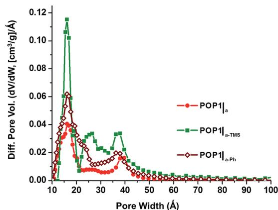
Fig. 4 Pore size distributions based on DFT calculations (slit-pore model) for  $\text{POP1}|_{\text{a}}$  (red circles),  $\text{POP1}|_{\text{a-TMS}}$  (green squares), and  $\text{POP1}|_{\text{a-Ph}}$  (brown diamonds).
