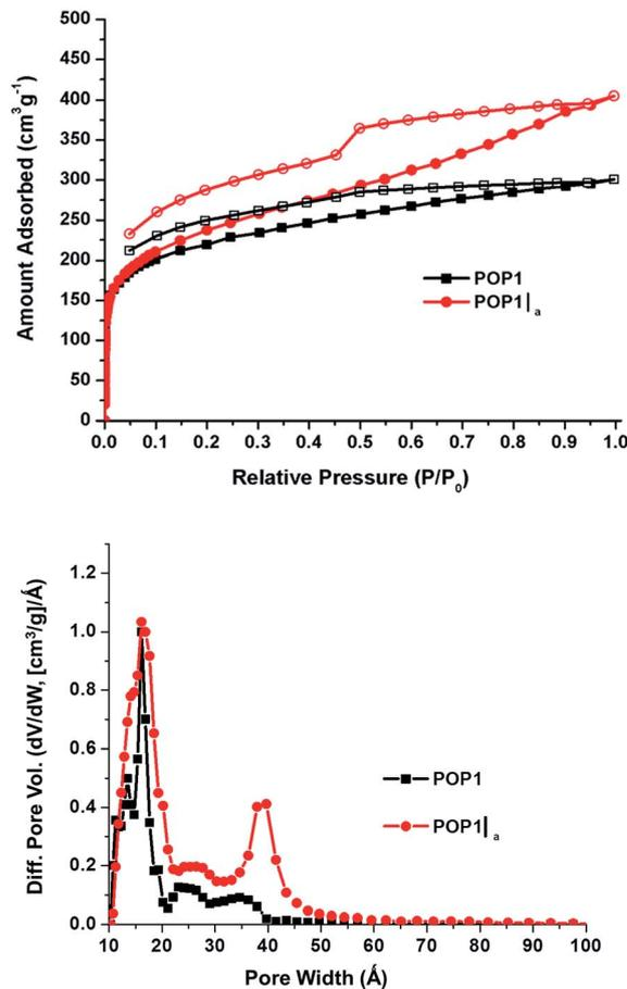
Fig. 2 (Top) N<sub>2</sub> isotherms, measured at 77 K, of POP1 (black squares) and POP1<sub>a</sub> (red circles). Closed symbols, adsorption; open symbols, desorption. (Bottom) Pore size distributions based on DFT calculations (slit-pore model) for POP1<sub>a</sub> (red circles) and POP1 (black squares).
