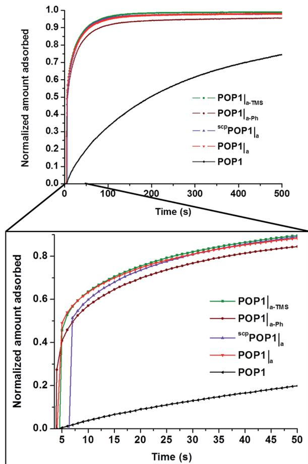
Fig. 6 Time-dependent propane-uptake profiles for POP1, POP1<sub>|a</sub>, scpPOP1<sub>|a</sub>, POP1<sub>|a-TMS</sub>, and POP1<sub>|a-Ph</sub> at 0.3 bar and 298 K. Data in each profile were normalized to the maximum uptake values at 15 000 s (see complete set of data in the ESI,† Fig. S13).
