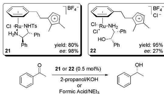
**Scheme 8** Ionophilic ruthenium complex-catalysed transfer hydrogenation reactions.
