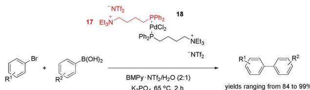
Scheme 5 PdCl<sub>2</sub>-tagged phosphine used as a precursor in the Suzuki cross-coupling reaction.
