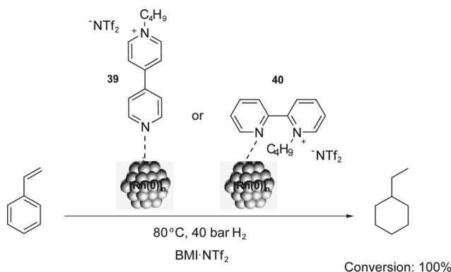
Scheme 18 Hydrogenation of styrene catalysed by [Rh(0)]<sub>n</sub> NPs, which are stabilised by the bipyridinium CTLs 39 and 40.
