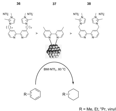
Scheme 17 Hydrogenation of arenes, catalysed by [Rh(0)]<sub>n</sub> NPs stabilised by CTLs in ILs, and the activity observed for the different ligands.
