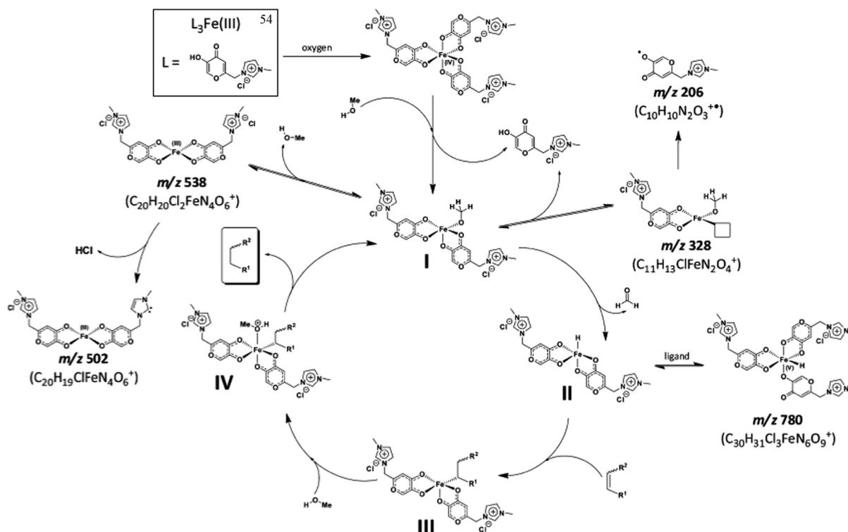
Scheme 30 Proposed catalytic cycle for olefin reduction catalysed by 54 in the presence of methanol. Major ions detected in the ESI(+)-QTOF-MS experiments are indicated by their *m/z* values, and proposals for the origins of the intermediates are shown. Reprinted with permission from ref. 112. Copyright (2012) American Chemical Society.
