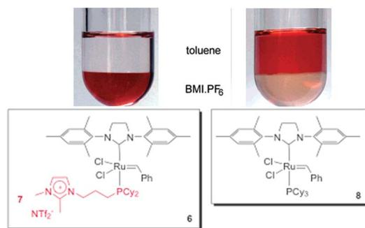
Fig. 1 Comparison of the distribution of **6** and **8** in a biphasic system composed of BMI·PF<sub>6</sub> and toluene. Adapted from ref. 24. Copyright (2008) American Chemical Society.
