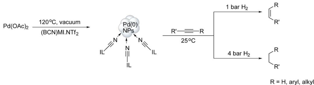
Scheme 20 Hydrogenation of alkynes, which is controlled by a variable hydrogen gas pressure.<sup>60</sup>
