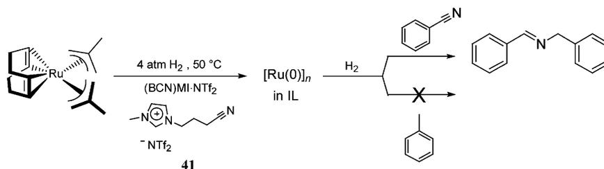
Scheme 19 Selective hydrogenation of benzonitrile, catalysed by  $[\text{Ru}(0)]_n$  NPs in a nitrile-functionalised IL.<sup>54</sup>
