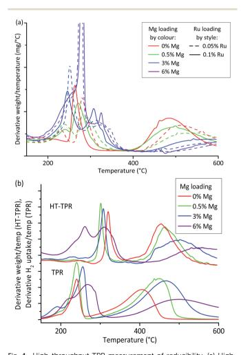
Fig. 4 High-throughput TPR measurement of reducibility. (a) High-throughput TGA in 5%  $\rm H_2$  acts as a high-throughput TPR (HT-TPR) screen to assess reducibility for OoA 1 samples. Mg lowers reducibility while Ru increases it. (b) Comparison of HT-TPR and conventional TPR traces for the scaled up samples showing that both methods show the same features, but these are shifted around 75 °C to higher temperatures in the case of the HT-TPR traces.
