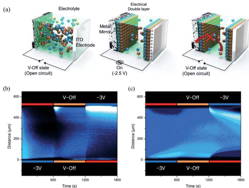
Fig. 3 (a) Schematic diagram of the ion distribution in the transparent state, reflective state, and V-off state. *In situ* fluorescence intensities between two ITO electrodes visualized by analyzing the confocal microscopic intensities over time, for (b) TITBAB and (c) TIBEIB with pyrene as a fluorophore to trace the ion transport ( $\lambda_{\text{exi}} = 405 \text{ nm}$ ). The light blue region indicates a high concentration of pyrene- $\text{Ag}^+$ .
