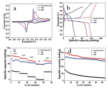
Fig. 5 The electrochemical properties of NaVPO<sub>4</sub>F precursor and NaVPO<sub>4</sub>F sintered at 750 °C and 800 °C: (a) cyclic voltammograms at a scan rate of 0.1 mV s<sup>-1</sup>; (b) the typical first cycle profiles of charge–discharge curves at 0.1 C; (c) performance at various rates from 0.1 C to 1 C; (d) cycle performances at 0.1 C.
