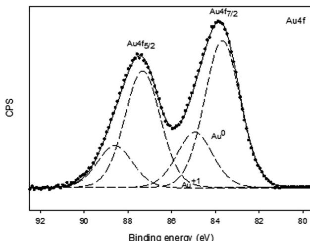
Fig. 8 XPS spectra in the Au 4f region of Au@UiO-66-NaBH<sub>4</sub> after catalysis.
