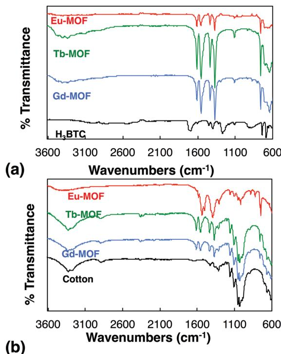
Fig. 7 FTIR spectra of (a) H<sub>3</sub>BTC and Ln-MOFs solids, and (b) clean cotton and Ln-MOFs grown on cotton fibers.
