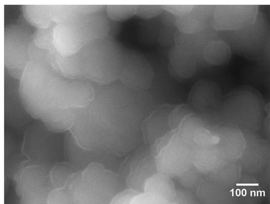
Fig. 5 SEM image of the fracture surface of a Cu fine particle pellet pressed at 100 °C. Cu fine particles are covered by BDVE polymer residues.
