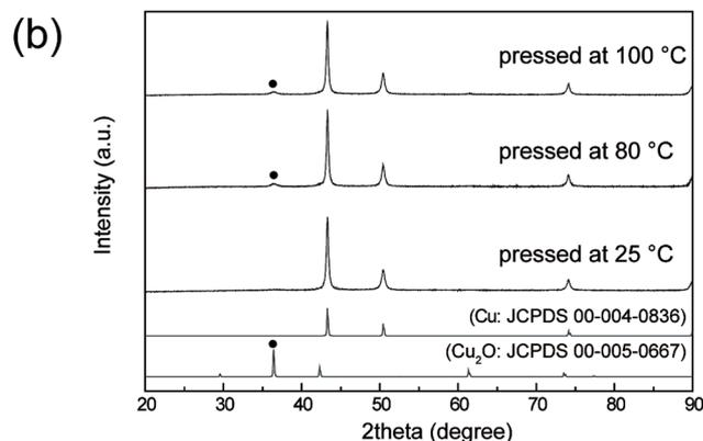
Fig. 4 (a) Resistivities of hot-pressed Cu pellets with (circles: ●) and without (triangles: ▲) BPMS as the thermal acid generator. The resistivity of bulk copper is  $1.7 \times 10^{-6} \text{ } \Omega \text{ cm}$  and is displayed as the dashed line. (b) XRD patterns of hot-pressed Cu pellets with BPMS. The (111) plane of  $\text{Cu}_2\text{O}$  is marked as closed circle (●).
