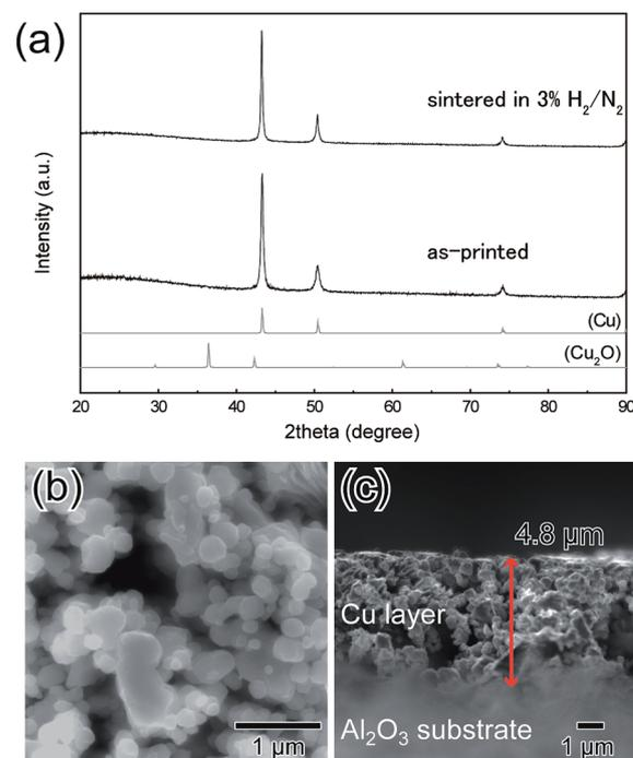
Fig. 7 (a) XRD patterns of Cu films on a glass before and after sintering. (b) SEM image of the Cu film sintered at 150 °C in 3% H<sub>2</sub> in N<sub>2</sub> gas. (c) Cross-sectional SEM image of (b). The thickness of film was 4.8 μm marked as red arrowed line.
