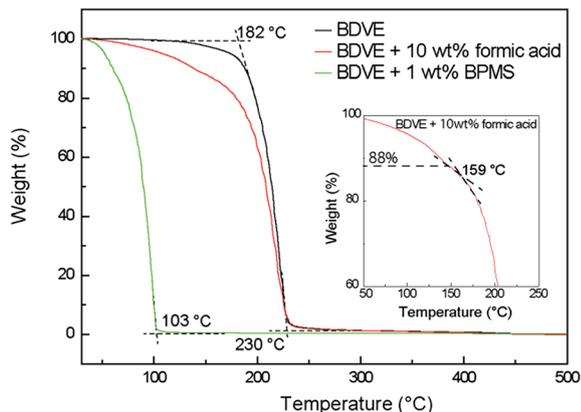
Fig. 3 TGA charts of BDVE with and without acids. TG measurements were carried out under air flow ( $200 \text{ cm}^3 \text{ min}^{-1}$ ) at the heating rate of  $1 \text{ }^\circ\text{C min}^{-1}$ . (black line) BDVE without acids. (red line) BDVE with 10 wt% of formic acid. (green line) BDVE with 1 wt% of BPMS. (Inset) Magnified curve of BDVE with 10 wt% of formic acid.
