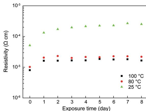
Fig. 6 Corrosion tests of the hot-pressed conductive Cu pellets with BPMS. The condition of the test was 85 °C and 85% relative humidity. The resistivities were increased after 1 day in the condition. However, the resistivities lasted for other 7 days without any obvious increase.
