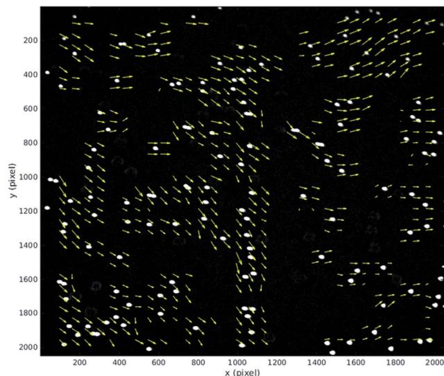
Fig. 7 Displacement vector field of 10  $\mu\text{m}$  fluorescent beads during a mirror cycle over the full field of view (1 Hz mirror cycle frequency). The vectors are scaled, with the average vector approximately 2 pixels long. The vectors highlight both mean motion from imperfect device alignment, and spatial variation resulting from acoustic causes. The flow direction is along the y-axis.
