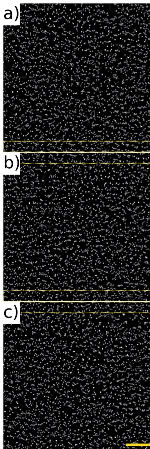
Fig. 11 Fluorescent beads (10  $\mu\text{m}$ ) recorded at  $104 \text{ mm s}^{-1}$ , 80 fps. Average throughput of 208 800 beads per second. (a–c) Represent a sample of three consecutive frames, the dotted regions highlight an overlap between frames of 140 pixels which can be adjusted by changing the amplitude of the signal driving the galvo mirror. Image size  $2048 \times 2048$ , field of view  $1.3 \times 1.3 \text{ mm}$ . Scale bar  $200 \mu\text{m}$ .
