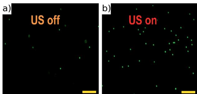
Fig. 4 Fluorescent 10  $\mu\text{m}$  beads flowing in the channel with acoustic focussing deactivated (a), and activated (b). These images are taken at low flow rates, and no galvo mirror tracking to illustrate the requirement for acoustic focussing. A movie of this can be found in ESI.† Scale bars 100  $\mu\text{m}$ .
