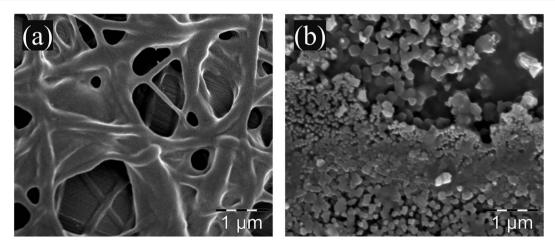
SEM images of the PVA-EA 3:1 nanofibres after the PVA matrix was removed at (a) 150 °C and (b) RT.
