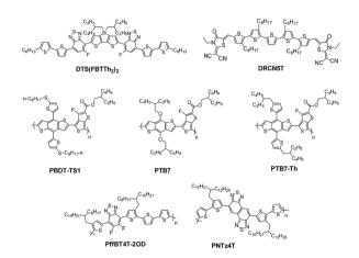
Fig. 2 The molecular structures of typical small-molecule and polymer donors from which a PCE of 10-11% or 11-12% has been realized for single-junction or tandem solar cells. The molecules are reported as follows: PTB7 ( $E_g^{\rm opt}=1.63~{\rm eV}$ ),  $^{22}$  PTB7-Th (1.58 eV),  $^{23}$  DTS(FBTTh<sub>2</sub>)<sub>2</sub> (1.55 eV),  $^{24}$  DRCN5T (1.60 eV),  $^{25}$  PBDT-TS1 (1.51 eV),  $^{26}$  PffBT4T-2OD (1.55 eV),  $^{5}$  and PNTz4T (1.54 eV).  $^{34}$
