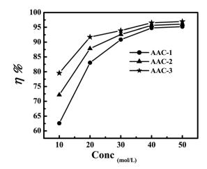
Fig. 2 Variation of inhibition efficiency with AACs concentration.
