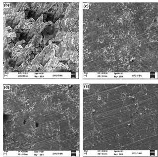
Fig. 8 (a-e) SEM images of mild steel surfaces: (a) abraded, (b) in absence of AACs and in the presence of 40 mg  $L^{-1}$  of (c) AAC-1, (d) AAC-2, and (e) AAC-3.
