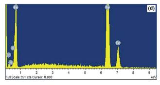
Fig. 9 (a-d) EDX images of mild steel: (a) in absence of AACs and in the presence of 40 mg  $L^{-1}$  of (b) AAC-1, (c) AAC-2, and (d) AAC-3.
