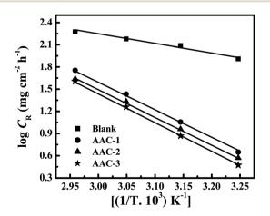
Fig. 3  $\,$  Arrhenius plots for the corrosion rate of mild steel  $\it versus$  the temperature in 1 M HCl.
