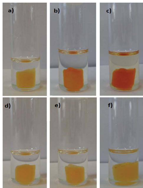
Fig. 6 TOCNF2-**bPEI-Sens** (10%) in DMSO (a), (TBA)F  $0.05\text{ M}$  (b), (TBA)F  $0.5\text{ M}$  (c), (TBA)Cl  $0.5\text{ M}$  (d), (TBA)AcO  $0.5\text{ M}$  (e), (TBA)H<sub>2</sub>PO<sub>4</sub>  $0.5\text{ M}$  (f). Temperature:  $55\text{ }^\circ\text{C}$ . Contact time:  $30\text{ min}$ .
