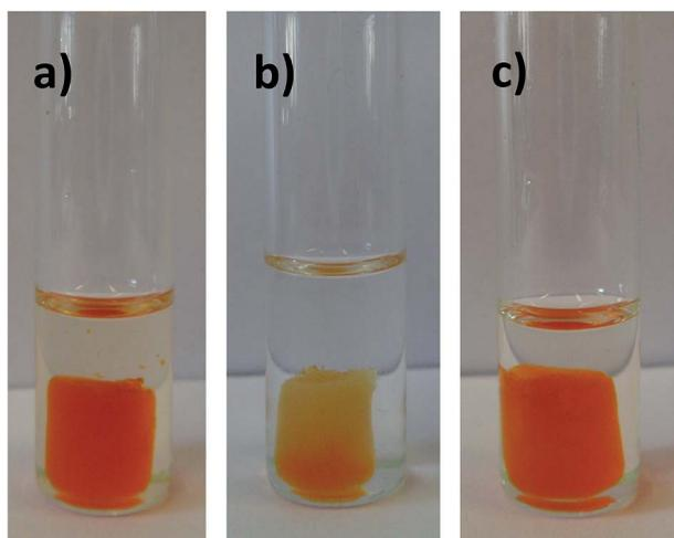
Fig. 8 TOCNF2-bPEI-Sens (10%) in TBAF 0.5 M (DMSO) (a), during its regeneration in MeOH (b) and final reuse in TBAF 0.5 M (DMSO) (c). Temperature: 55 °C. Contact time: 30 min.
