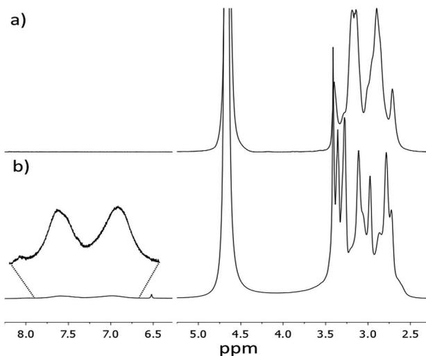
Fig. 1 <sup>1</sup>H-NMR spectra of: (a) **bPEI**; (b) **bPEI-Sens** (10%). Solvent: D<sub>2</sub>O + CF<sub>3</sub>COOH, T = 23 °C.
