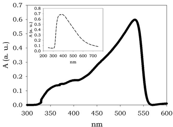
Fig. 7 Reflectance spectrum of TOCNF2-bPEI-Sens (10%) after immersion into a solution of (TBA)F 0.5 M,  $A_{\max} = 532$  nm; the spectrum of DMSO-wet TOCNF2-bPEI-Sens (10%) was taken as baseline; inset: spectrum of the TOCNF2-bPEI-Sens (10%),  $A_{\max} = 392$  nm.
