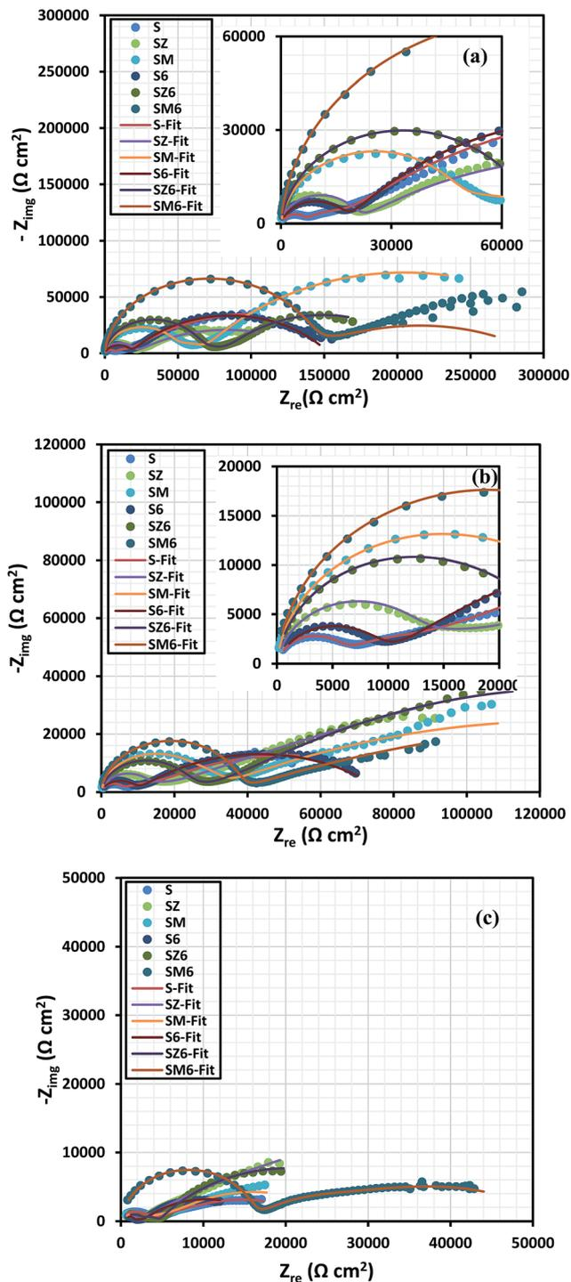
Fig. 4 Nyquist plot of experimental data for all coating matrices after (a) 24 hours (b) 48 hours, and (c) 2 weeks of immersion in 3.5 wt% NaCl solution (insert: Nyquist curves showing  $Z$  values at higher frequencies).
