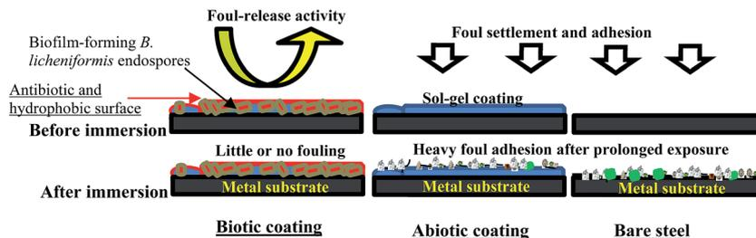
**Scheme 1** Foul-releasing mechanism in the presence of the endospores of thermophilic *B. licheniformis* strain in the sol-gel coating involves surface resistance towards foul settlement and adhesion due to the formation of bacterial biofilm with an antibiotic character.
