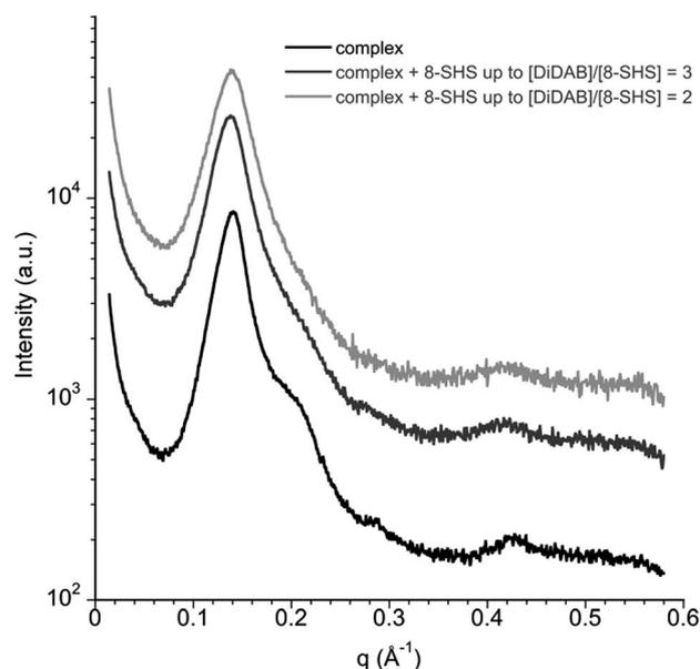
**Fig. 6** SAXS spectra of DNA/DiDAB/8-SHS precipitates at  $R = 0.85$ , at 25.0 °C. The initial [DiDAB]/[8-SHS] mole ratio was 4 (black line). 8-SHS was added to reach a [DiDAB]/[8-SHS] final ratio equal to 3 (grey line) and 2 (light grey line).
