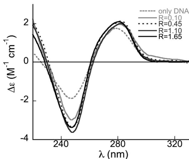
**Fig. 5** CD spectra reported as  $\Delta\epsilon$  ( $M^{-1} \text{ cm}^{-1}$ ) for DiDAB/8-SHS/DNA complexes at  $R = 0.10$  (light grey line), 0.45 (grey dotted line), 1.10 (grey line) and 1.65 (black line). All spectra are compared with that of calf thymus DNA in water (light grey dotted line). Measurements were run at 25.0 °C. Spectra were normalized per nucleotide concentration.
