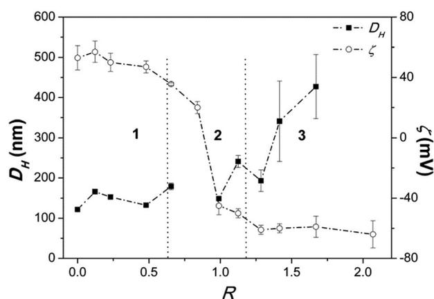
Fig. 1  $D_H$  (nm), (■), and  $\zeta$  (mV), (○), vs. the charge ratio  $R = [\text{PO}_4^-]/[\text{DiDA}^+]$  for DiDAB/8-SHS vesicles and DNA. The interpolating lines are drawn as a guide for the eye. The three regions are indicated and separated by dotted lines. Measurements were run at 25 °C. Error bars represent standard deviations.
