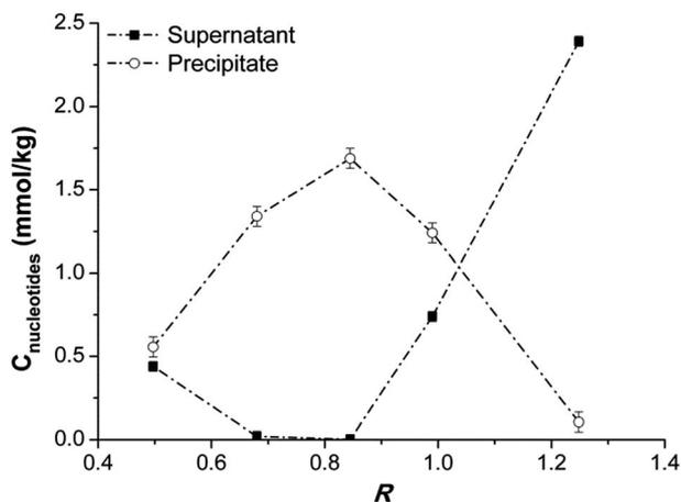
Fig. 2  $C_{\text{nucleotide}}$  (mmol kg<sup>-1</sup>) vs.  $R$  ( $[\text{PO}_4^-]/[\text{DiDA}^+]$ ) in the supernatant (■) and in the precipitate (○). Measurements refer to 25 °C.  $C_{\text{nucleotide}}$  consists of the concentration of the DNA free in solution and that of the DNA in the complexes. Error bars represent standard deviations. The interpolating lines are guide to the eye.
