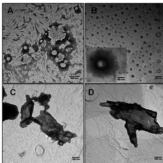
Fig. 3 TEM micrographs of DiDAB/8-SHS/DNA complexes in solution at charge ratio  $R =$  (A) 0, (B) 0.25, (C) 0.68 and (D) 1.00. In (A) artefacts are due to the presence of crystallized salts in the heterogeneous dispersion.
