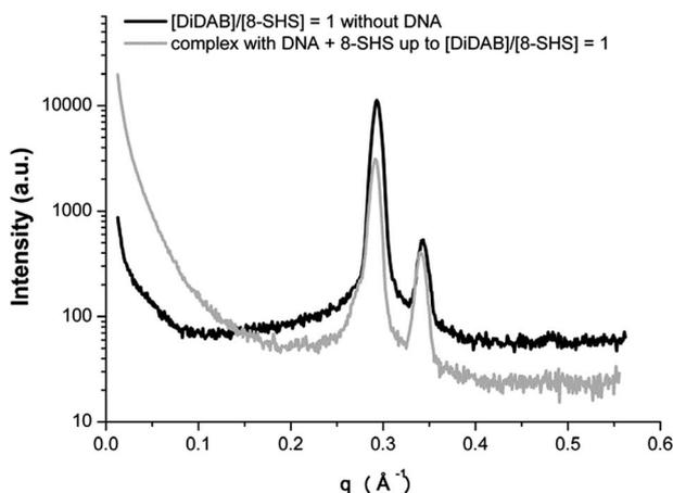
**Fig. 7** SAXS spectra of [DiDAB]/[8-SHS] equimolar complex (black line) and of the phase formed by adding 8-SHS to the DNA/DiDAB/8-SHS complex at  $R = 0.85$  up to a [DiDAB]/[8-SHS] final ratio equal to 1 (grey line). Measurements were run at 25.0 °C.
