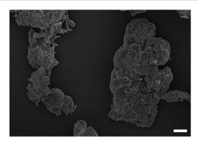
Fig. 1 Examples of SEM image of PMMA wear debris. Bar correspond to 1 microns.
