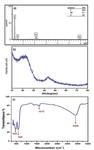
Fig. 5 (a) EDX analysis, (b) XRD pattern and (c) FTIR spectrum of  $\rm MnO_2\text{-}NP\text{-}AC$ .
