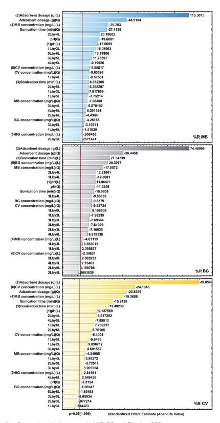
Fig. 7 Standardized main effect Pareto chart for the removal of MB, BG and CV using CCD.
