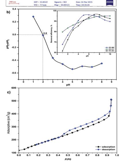
Fig. 4 (a) FESEM image of the prepared  $MnO_2$ -NP-AC, (b) pHzpc of  $MnO_2$ -NP-AC (pH $_i$  = initial pH and pH $_f$  = final pH) and (c) nitrogen adsorption–desorption isotherms.
