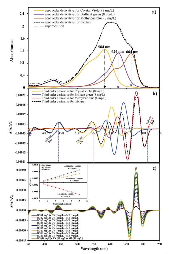
Fig. 3 (a) Zero order absorption spectra of CV, BG and MB in single and ternary solutions (with an initial dye concentration of 8 mg L<sup>-1</sup> for each dye). (b) Third order derivative spectra of CV, MG and MB in ternary solutions. (c) Calibration graph at 710 nm for MB, 550 nm for CV and 440 nm for BG.
