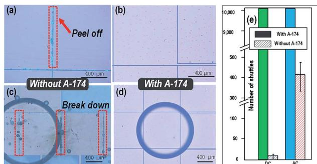
Fig. 5 Topographic images of DMF chips coated with Ta<sub>2</sub>O<sub>5</sub> and Parylene C with and without A-174 as an adhesion promoter. (a) Freshly fabricated chip without A-174. (b) Freshly fabricated chip with A-174. (c) After running droplets on chip without A-174, (d) After running droplets on chip with A-174.
