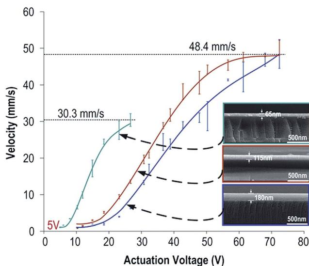
Fig. 6 Droplet transportation velocity as a function of the actuation voltage on chips with different thickness of Ta<sub>2</sub>O<sub>5</sub> layers. Insert: scanning electron microscope (SEM) cross-section micrographs of different thickness of Ta<sub>2</sub>O<sub>5</sub> thin films. The velocity was an average of a droplet moving across 12 electrodes. All experiments have been repeated for three times.
