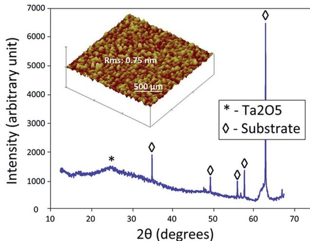
Fig. 3 X-ray diffraction (XRD) pattern of rapidly thermal annealed (RTA) Ta<sub>2</sub>O<sub>5</sub> thin film at 400 °C for 10 min in N<sub>2</sub> atmosphere. Insert: topographic image characterized by atomic force microscopy (AFM).
