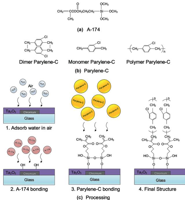
Fig. 4 Schematics of A-174 promoting adhesion between Ta<sub>2</sub>O<sub>5</sub> and Parylene C. (a) Chemical structure of A-174; (b) chemical structure of dimer, monomer and polymer Parylene-C; (c) bonding process of Ta<sub>2</sub>O<sub>5</sub> and Parylene-C.
