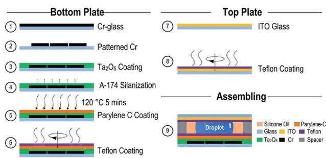
Fig. 1 Fabrication procedure of Ta<sub>2</sub>O<sub>5</sub> and Parylene C insulated two-plate DMF chip.
