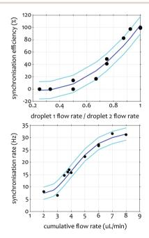
Fig. 5 (a) Dependence of synchronization performance on droplet size difference. A synchronization efficiency above 95% is only achieved if the two synchronized droplet types enter the chamber at equal flow rates. (b) Dependence of the synchronization rate on total flow rate, showing that throughput increases as a function of flow rate.
