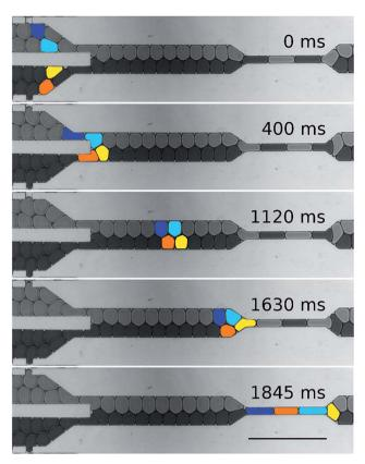
Fig. 2 A series of images extracted from a high-speed video (Movie S1†) showing a set of droplets moving through the synchronization architecture (scale bar – 600 μm). Droplets are passively ordered into an A-B alternating pattern when they are injected into the common channel (400 ms into the video). Once this channel is constricted so as to only allow a single file of droplets (1600 ms into the video) the two rows of droplets are impelled into an A-B sequential order.
