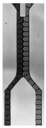
Fig. 6 Splitting a stream of synchronized droplets in an A-B alternate configuration into its constituent droplets and recombination of the separated streams. Direction of flow is from top to bottom (indicated by the arrow). This produces a situation where a uniform of droplets are flowing through the individual channel, but where each side contains droplets of different composition.
