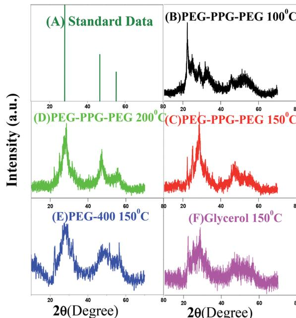
Fig. 1 P-XRD of BIZS prepared at various temperature and solvent.
