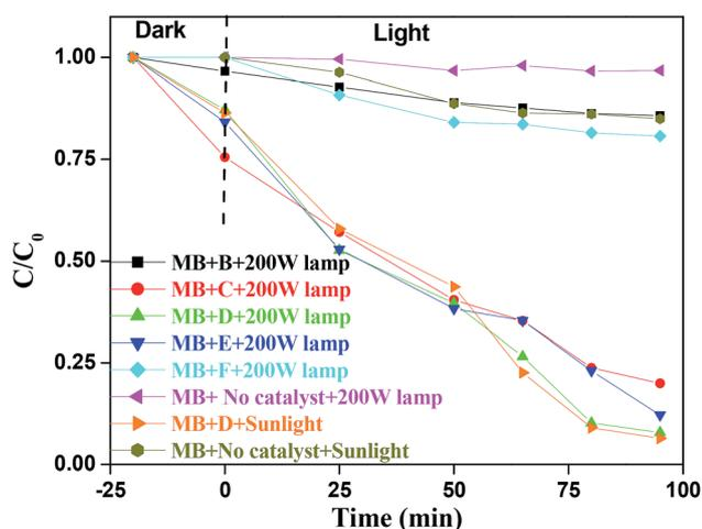
Fig. 10 Photodegradations of MB, ( $C/C_0$ ) versus irradiation time under visible light.
