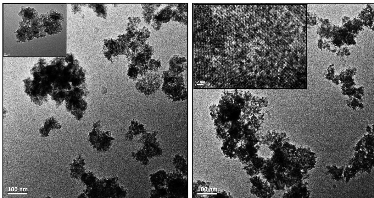
Fig. 4 TEM image of BIZS (sample D) at different magnification.
