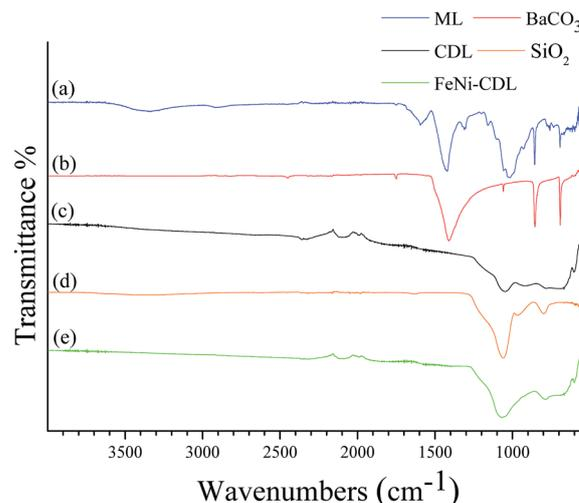
Fig. 2 IR spectra of the mineralized lignin (a), of  $\text{BaCO}_3$  (b), of the carbonized/demineralized lignin (c), of  $\text{SiO}_2$  (d), and of the carbonized/demineralized lignin impregnated with the salt precursors of Fe and Ni and then heat-treated at  $800\text{ }^\circ\text{C}$  for 2 h under  $\text{N}_2$  (e).
