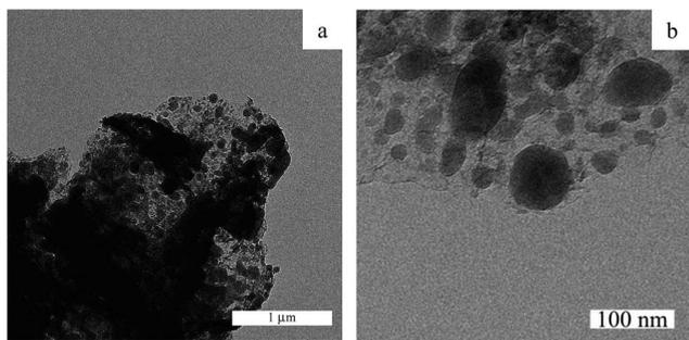
Fig. 5 Low (a) and high (b) magnification TEM images of the carbonized/demineralized lignin impregnated with the salt precursors of Fe and Ni and then heat-treated at 800 °C for 2 h under N<sub>2</sub>.
