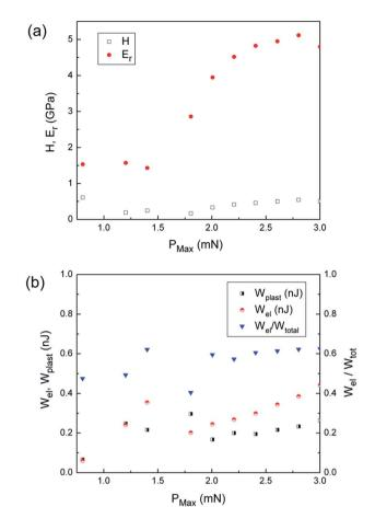
Fig. 4 Values of (a) hardness and reduced Young's modulus and (b) indentation energies and elastic recovery ( $W_{\rm el}/W_{\rm tot}$ ) of the complex.
