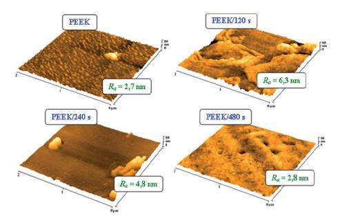
Fig. 1 AFM images of pristine polyetheretherketone [PEEK] and PEEK treated by Ar plasma for 120, 240 and 480 s [PEEK/120 s; PEEK/240 s; PEEK/480 s]. R<sub>a</sub> is average surface roughness in nm.
