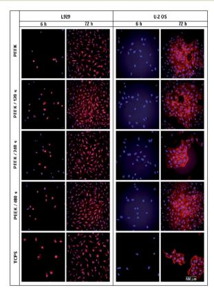
Fig. 4 Fluorescence microscopy images of L929 and U-2 OS cells adhered (6 h) and proliferated (72 h) on treated polyetheretherketone [PEEK] scaffolds in the following order: pristine polymer [PEEK], plasma treated [120, 240 and 480 s] and tissue culture polystyrene [TCPS]. Cell cytoskeleton labeled with phalloidin-Atto 565 and cell nuclei with DAPI. The scale bar of all images corresponds to 100 µm.
