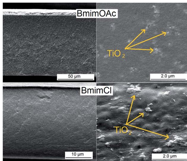
Fig. 3 Scanning electron microscopy images (left: cross-section; right: top view) of cellulose– $\text{TiO}_2$  P90 (ratio: 20 : 1) nanocomposite films from 10 wt% cellulose solutions in ionic liquid. (note the different magnification for the material prepared from BmimCl).
