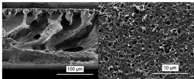
Fig. 7 Scanning electron microscopy images (left: cross-section; right: top view) of cellulose acetate–TiO<sub>2</sub> P90 (ratio: 10 : 1) membrane prepared by phase separation from a DMF solution.
