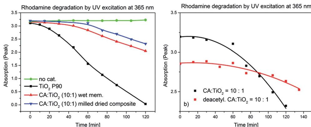
Fig. 8 (a) Rhodamine B degradation with different photocatalytically active materials; (b) rhodamine B degradation cellulose acetate–TiO<sub>2</sub> P90 (ratio: 10 : 1) milled dried composite and corresponding regenerated cellulose–TiO<sub>2</sub> P90 (ratio: 10 : 1) milled dried composite.
