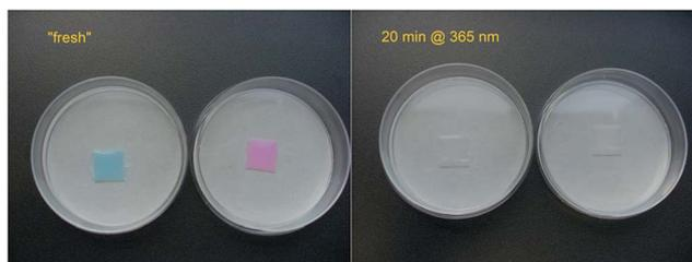
Fig. 4 Photocatalytic degradation of methylene blue and rhodamine B on cellulose–TiO<sub>2</sub> P90 (ratio: 10 : 1) nanocomposite films from ionic liquid solutions.
