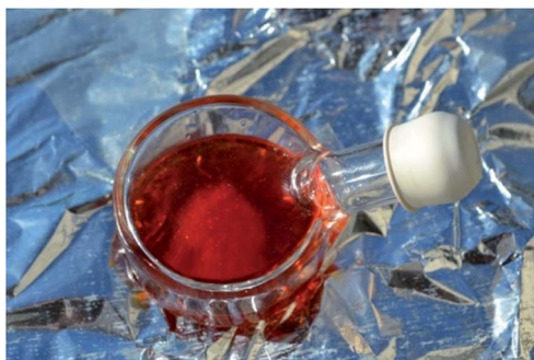
Fig. 1 Pyrex glass vessel (20 mL capacity) used for the sunlight synthesis of picenes 2a–c . As shown, the product precipitated out upon prolonged exposure to solar radiation.
