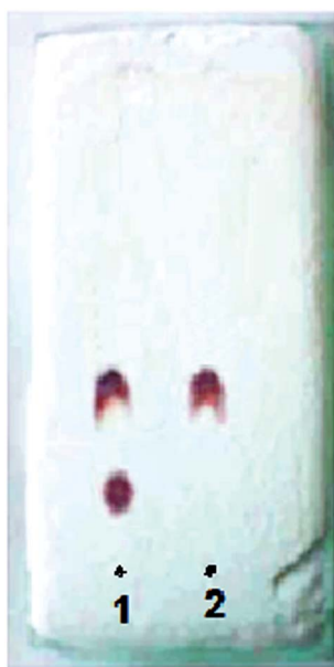
Fig. 2 Photograph of an actual chromatogram showing resolution of ( \pm )-SeMet. From left to right: Line 1, lower spot is of (-)-isomer and the upper spot is of (+)-isomer (resolved from the racemic mixture); Line 2, pure (+)-isomer. Mobile phase: CH 3 CN-CH 3 OH-CH 2 Cl 2 -H 2 O (10 : 1.5 : 0.5 : 1.5, v/v). Solvent front: 8 cm; temperature: 25 \pm 2 ^{\circ} C; detection: ninhydrin solution (0.3% in n -BuOH); development time: 10 min.
