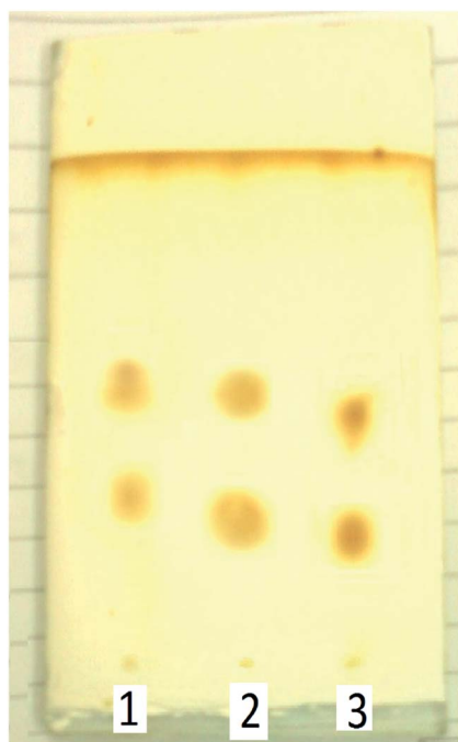
Fig. 4 Photograph of an actual chromatogram showing resolution of (±)-Atl, (±)-Orc and (±)-Bel. From left to right: Line 1, 2 and 3, respectively, for (±)-Orc, (±)-Bel and (±)-Atl, lower spot is of (–)-isomer, and the upper spot is of (+)-isomer (resolved from the racemic mixture). Mobile phase: \text{CH}_3\text{CN}-\text{CH}_3\text{OH}-\text{CH}_2\text{Cl}_2-\text{H}_2\text{O} (6 : 3 : 3 : 1.5, v/v). Solvent front: 8 cm; temperature: 25 \pm 2^\circ\text{C} ; detection: iodine vapor; development time: 10 min.
