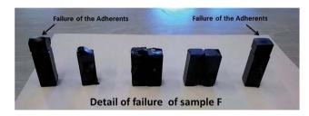
Fig. 8 Detail of failure in sample F.
