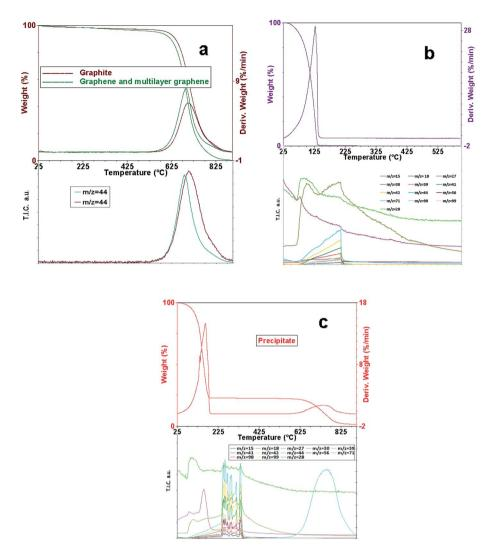
Fig. 6 TG-DTG and relevant total ion current signals of graphite and G + MLG (a). TG-DTG and relevant total ion current signals of NMP (b). TG-DTG and relevant total ion current signals of the precipitate (c).
