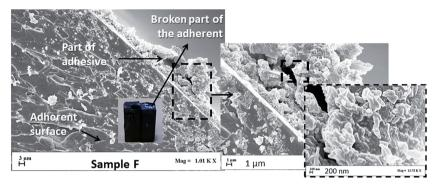
Fig. 13 FESEM micrograph of the fracture surfaces of the bonding areas of sample F. Failure in tensile test and detail of the magnifications of the neighboring region.
