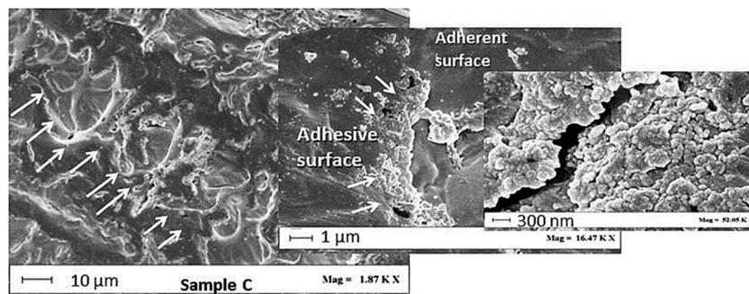
Fig. 10 FESEM micrograph of the fracture surfaces of the bonding areas of sample C. Failure in tensile test and detail of the magnifications of the neighboring region.
