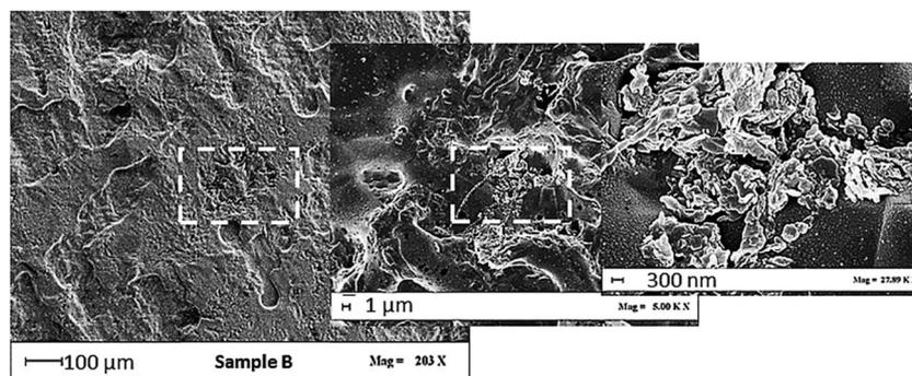
Fig. 9 FESEM micrographs of the fracture surfaces of the bonding areas of sample B. Failure in tensile test and detail of the magnifications of the neighboring region.
