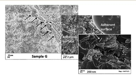
Fig. 14 FESEM micrograph of fracture surfaces of the bonding areas of sample G. Failure in tensile test and detail of the magnifications of the neighboring region.
