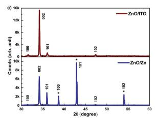
Fig. 1 SEM images of (a) ZnO/ITO and (b) ZnO/Zn nanorods (c) XRD patterns of the respective nanorods.
