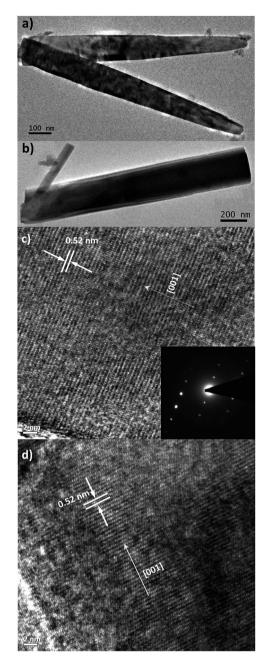
Fig. 2 Low-resolution TEM images of (a) ZnO/ITO and (b) ZnO/Zn nanorods. High-resolution TEM images of (c) ZnO/ITO and (d) ZnO/Zn nanorods. Inset shows the SAED pattern of ZnO/ITO nanorods.
