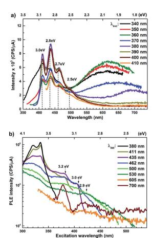
Fig. 6 (a) Excitation dependent PL spectra and (b) PLE spectra for different emission wavelengths of ZnO/Zn nanorods.
