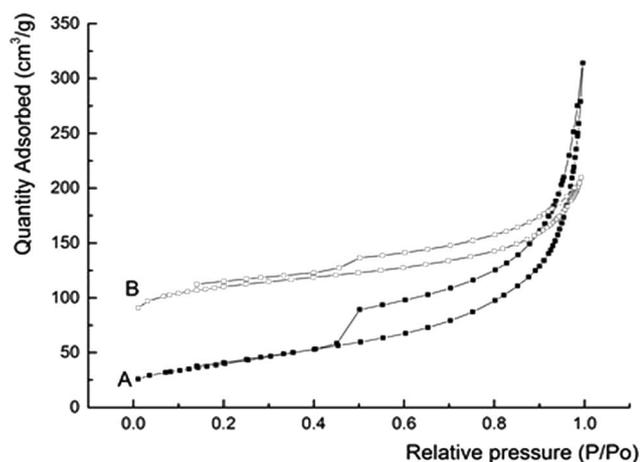
Fig. 8 Nitrogen adsorption–desorption isotherms for A – bare carbon monolith (prepared without the addition of carbon nanoparticles for comparative purposes) and B – carbon on carbon monolithic composite containing carbon onions.
