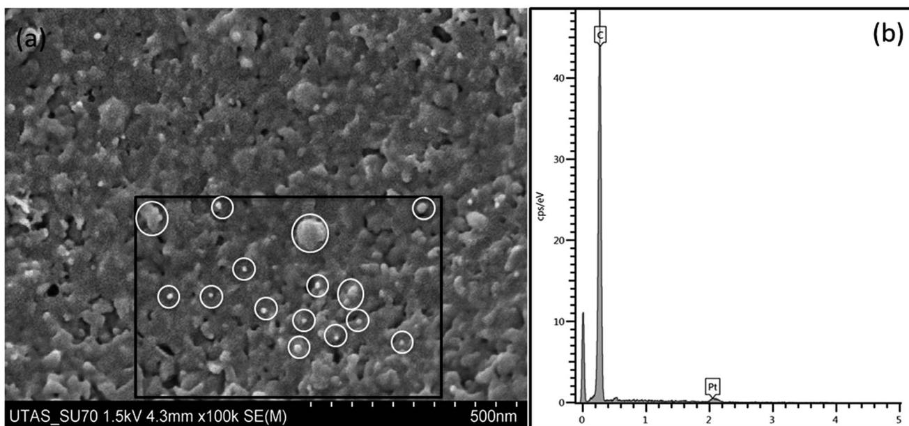
Fig. 4 (a) High magnification ( $\times 100\text{K}$ ) image of the wall of monolith macropore, showing the presence of a mesoporous structure (with surviving surface detonation nanodiamonds highlighted between 10 and 100 nm). (b) EDX spectrum for carbon monolith showing presence of carbon only (Pt from sputter coating).
