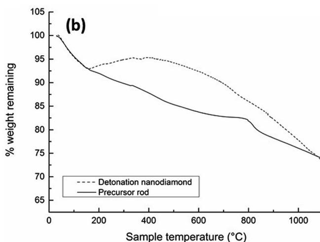
Fig. 2 (a) SEM image taken of a cross section of the precursor rod containing silica particles, and detonation nanodiamond (DND), before carbonisation at 1250 °C. (b) Thermogravimetric analysis curves for DND, and precursor rod containing the resorcinol–formaldehyde resin, with Fe<sup>3+</sup> catalyst, silica particles, and DND.
