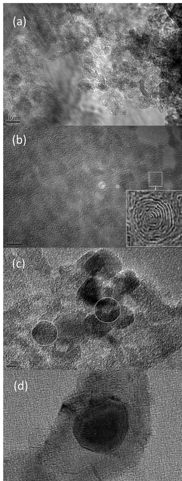
Fig. 5 TEM images of porous graphitic carbon composites. (a) Amorphous carbon, (b) carbon onions resulting from the thermal annealing of detonation nanodiamond (DND) under N<sub>2</sub> at 1250 °C, (c) DND remains intact within the porous graphitic carbon composite following pyrolysis up to 900 °C, (d) DND showing surface graphitisation following pyrolysis up to 900 °C.
