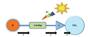
Fig. 4 Schematic drawing of donor- $\pi$ -bridge-acceptor organic sensitizers and their electron transfer processes under illumination.
