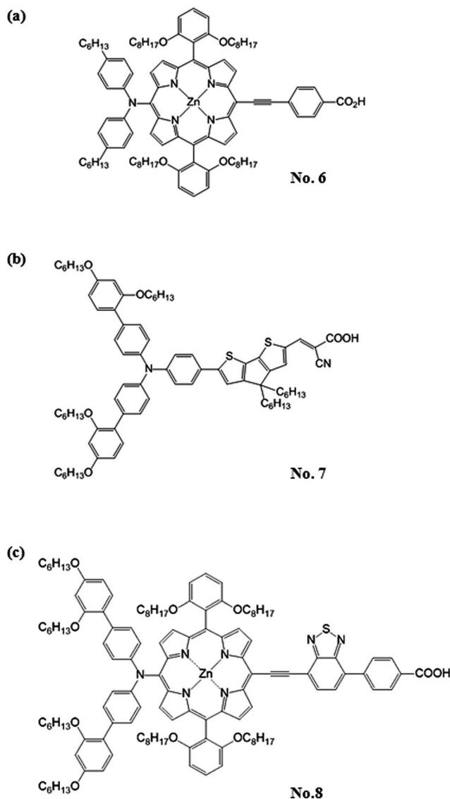
Fig. 3 The structure of (a) YD2-*o*-C8 sensitizer (No. 6), (b) Y123 sensitizer (No. 7) and (c) SM315 sensitizer (No. 8).
