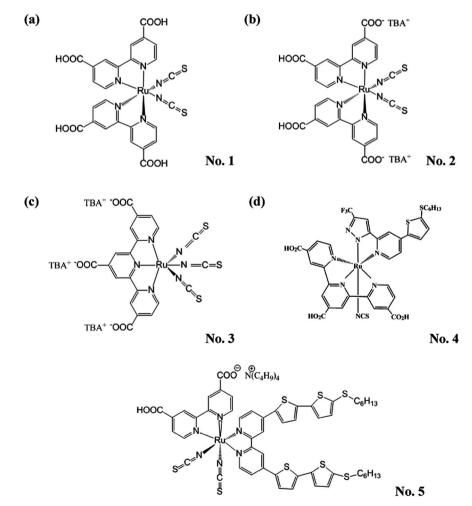
Fig. 2 The structures of partial ruthenium (Ru) complexes. (a) N3 (No. 1), (b) N719 (No. 2), (c) black dye (No. 3), (d) PRT-22 (No. 4) and (e) CYC-B11 (No. 5).
