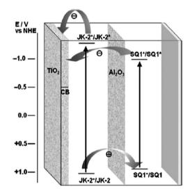
Fig. 9 Charge-transfer processes in multilayer co-sensitized  $\text{TiO}_2$  films with a  $\text{Al}_2\text{O}_3$  layer (CB = conduction band, NHE = normal hydrogen electrode). Reproduced by permission of The Royal Society of Chemistry.
