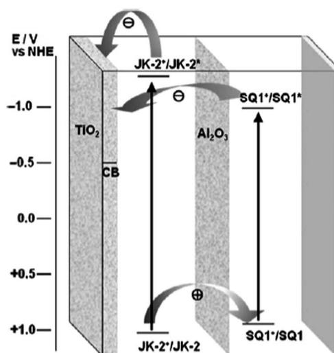
Fig. 9 Charge-transfer processes in multilayer co-sensitized TiO<sub>2</sub> films with a Al<sub>2</sub>O<sub>3</sub> layer (CB = conduction band, NHE = normal hydrogen electrode). Reproduced by permission of The Royal Society of Chemistry.
