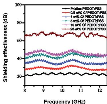
**Fig. 2** EMI shielding effectiveness as a function of frequency for the GNP/PEDOT:PSS composites with various GNP loadings.
