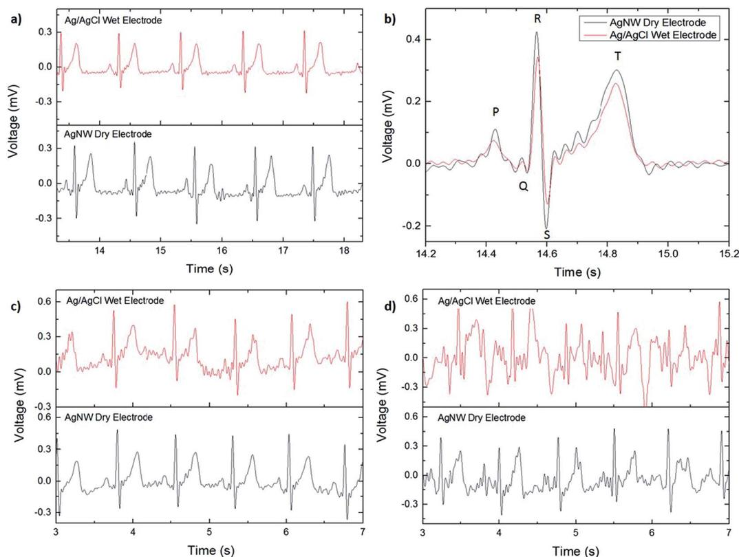
Fig. 3 (a) ECG recording of Ag/AgCl wet electrode and AgNW dry electrode taken while subject was seated and resting. (b) ECG signal comparison of the P, Q, R, S, and T waves between the Ag/AgCl electrode and NW electrode. (c) ECG signal comparison of the subject swinging their arms, one degree of movement. (d) ECG signal comparison of the subject jogging, two degrees of movement.
