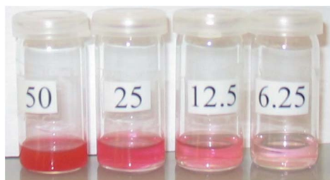
Fig. 3 Photograph of encapsulated Congo red by PG 2400 -PLA multiarm star copolymers with different [LA]/[OH] ratios at the same nanocarrier concentration.
