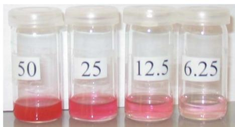
Fig. 3 Photograph of encapsulated Congo red by PG<sub>2400</sub>-PLA multiarm star copolymers with different [LA]/[OH] ratios at the same nanocarrier concentration.
