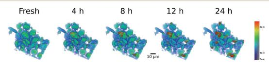
Fig. 12 Washcoat volume rendering illustrating the impact of aging time at 950 °C in static air.
