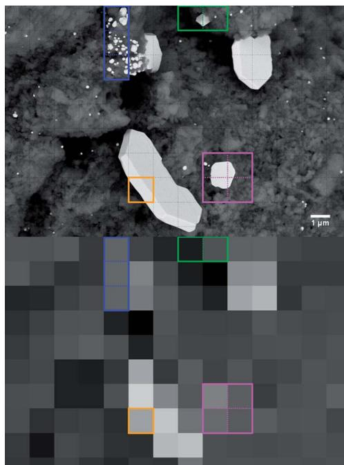
Fig. 6 Comparison of pixel and voxel sizes in SEM and μ-CT images relevant for data interpretation. (a) SEM image of a Pt/Al<sub>2</sub>O<sub>3</sub> sample (aged 24 h @ 950 °C) reveals various large platinum crystals. (b) Simulating the effect of 1.27 μm μ-CT voxel size by box averaging of (a).
