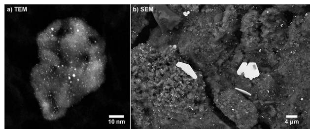
Fig. 3 (a) TEM image (STEM, 910k $\times$  magnification) of a fresh Pt/Al<sub>2</sub>O<sub>3</sub> sample. (b) SEM image (BSE, 8k $\times$  magnification) of a sample aged for 24 h at 950 °C.
