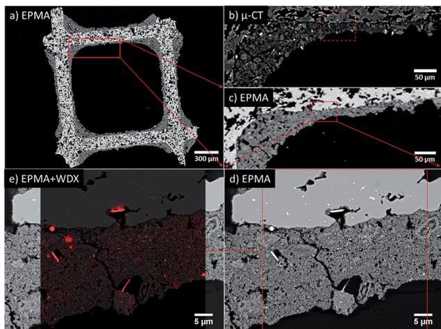
**Fig. 4** Mechanical cross section of an embedded sample, aged 24 h at 950 °C in static air, imaged by EPMA and  $\mu$ -CT. Back-scattered electron images of (a) the complete embedded honeycomb channel and (c) close up to the part containing the ROI box for the (d) high resolution EPMA with additional (e) WDX map of Pt overlaid. For comparison a (b)  $\mu$ -CT slice of the same sample part before embedding is shown with a dashed box indicating the ROI measured in (d and e).
