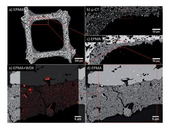
Fig. 4 Mechanical cross section of an embedded sample, aged 24 h at 950 °C in static air, imaged by EPMA and  $\mu\text{-CT}$ . Back-scattered electron images of (a) the complete embedded honeycomb channel and (c) close up to the part containing the ROI box for the (d) high resolution EPMA with additional (e) WDX map of Pt overlaid. For comparison a (b)  $\mu\text{-CT}$  slice of the same sample part before embedding is shown with a dashed box indicating the ROI measured in (d and e).
