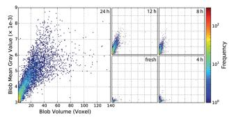
Fig. 11 2D histograms of blob mean gray values and volumes confirming the correlation of the plotted quantities. The main frame shows the state after 24 h aging at 950 °C and prior steps in the small frames. Frequencies are displayed using a logarithmic scale, see color bar.
