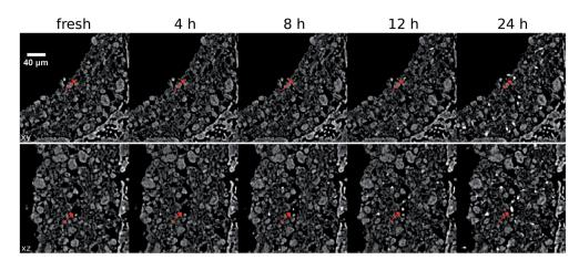
Fig. 5 Virtual cross sections through tomographic reconstructions for each aging step at 950 °C. Views are presented for planes along xy and xz. The magnification, 40  $\mu$ m scale bar, and gray scale are identical for all slices. Arrows indicate sintered features.
