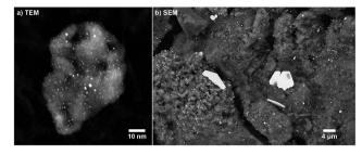
Fig. 3 (a) TEM image (STEM, 910k× magnification) of a fresh Pt/Al $_2O_3$  sample. (b) SEM image (BSE, 8k× magnification) of a sample aged for 24 h at 950 °C.
