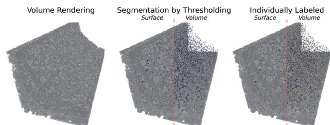
Fig. 8 Volume renderings of the analyzed honeycomb channel aged for 12 h at 950 °C. The segmentation yields all sintered voxels (blue) with high absorption, *i.e.* high Pt concentration, identical to bright regions in the left image. These are further separated into individually labeled blobs, indicated by different colors. Results of the last two steps are presented as view on surface and entire volume.
