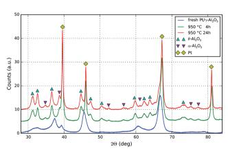
Fig. 2 Diffraction patterns of 4 wt% Pt/ $\gamma$ -Al $_2O_3$  powder: (a) fresh, (b) aged at 950 °C in static air for 4 h, and (c) aged for 24 h under the same conditions. Markers are added for metallic fcc phase of Pt ( $\spadesuit$ ),  $\theta$ -Al $_2O_3$  ( $\blacksquare$ ), and  $\alpha$ -Al $_2O_3$  ( $\blacksquare$ ) while  $\gamma$ -Al $_2O_3$  is the only detected phase in (a). The plots are unscaled and stacked for comparison.
