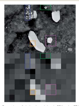
Fig. 6 Comparison of pixel and voxel sizes in SEM and  $\mu$ -CT images relevant for data interpretation. (a) SEM image of a Pt/Al<sub>2</sub>O<sub>3</sub> sample (aged 24 h @ 950 °C) reveals various large platinum crystals. (b) Simulating the effect of 1.27  $\mu$ m  $\mu$ -CT voxel size by box averaging of (a).
