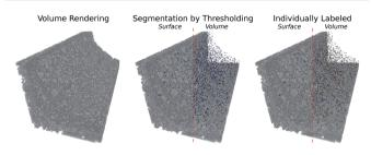
Fig. 8 Volume renderings of the analyzed honeycomb channel aged for 12 h at 950 °C. The segmentation yields all sintered voxels (blue) with high absorption, i.e. high Pt concentration, identical to bright regions in the left image. These are further separated into individually labeled blobs, indicated by different colors. Results of the last two steps are presented as view on surface and entire volume.
