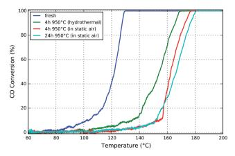
Fig. 1 Light-off curves for CO oxidation for honeycomb samples aged either (i) in static air for 4 and 24 hours, or (ii) with 10 vol% H<sub>2</sub>O in the gas stream for 4 hours
