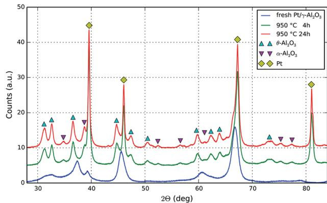
Fig. 2 Diffraction patterns of 4 wt% Pt/ $\gamma$ -Al<sub>2</sub>O<sub>3</sub> powder: (a) fresh, (b) aged at 950 °C in static air for 4 h, and (c) aged for 24 h under the same conditions. Markers are added for metallic fcc phase of Pt (◆),  $\theta$ -Al<sub>2</sub>O<sub>3</sub> (▲), and  $\alpha$ -Al<sub>2</sub>O<sub>3</sub> (▼) while  $\gamma$ -Al<sub>2</sub>O<sub>3</sub> is the only detected phase in (a). The plots are unscaled and stacked for comparison.
