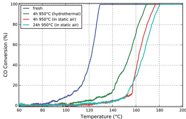
Fig. 1 Light-off curves for CO oxidation for honeycomb samples aged either (i) in static air for 4 and 24 hours, or (ii) with 10 vol% H<sub>2</sub>O in the gas stream for 4 hours.
