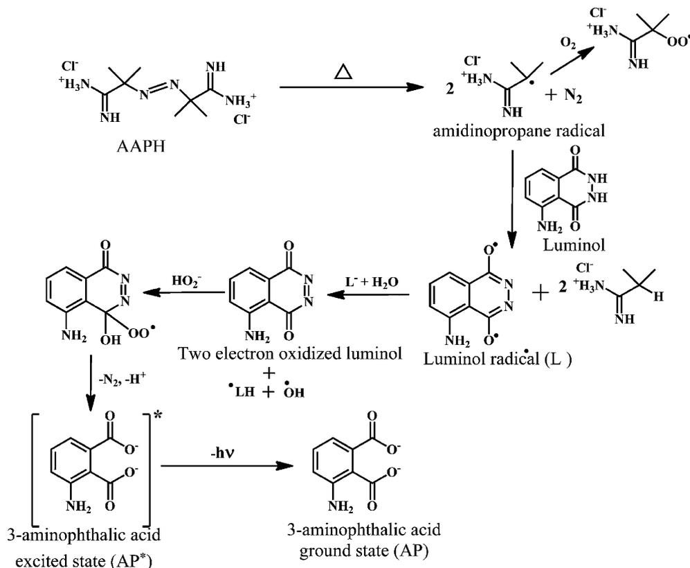
Scheme 20 Mechanism of AAPH induced chemiluminescence of luminol.
