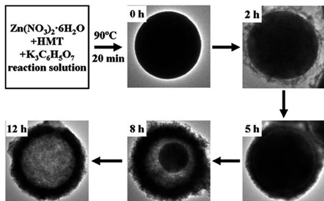
Fig. 6 Morphology evolution for zinc citrate microspheres with aging time (reprinted with permission from ref. 117; Copyright 2012 @ Royal Society of Chemistry).
