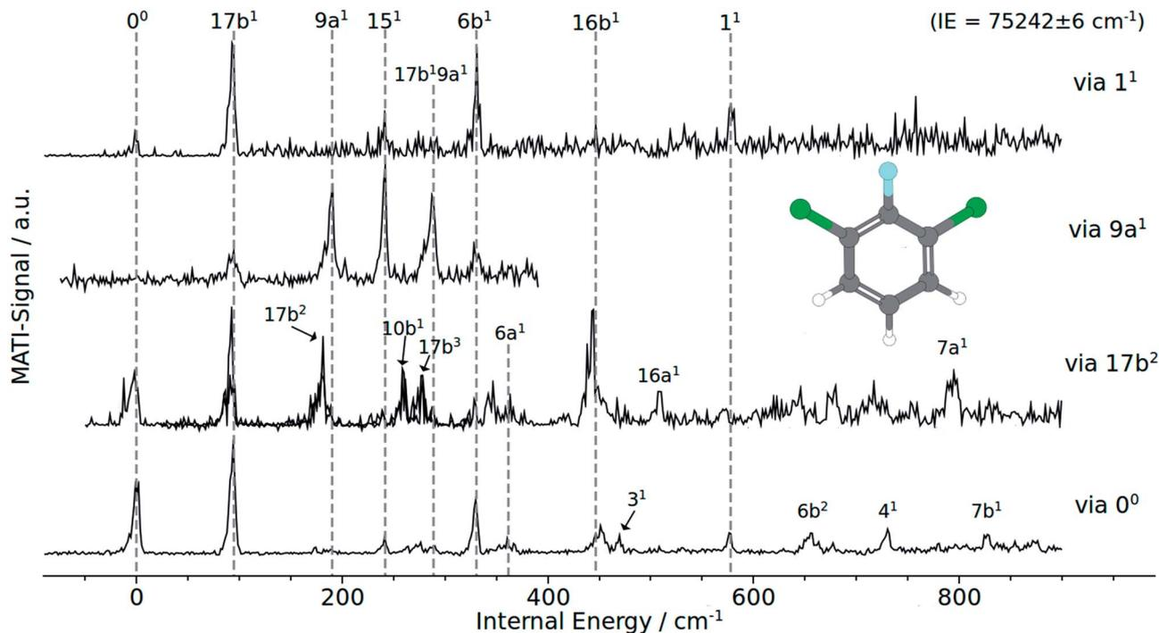
Fig. 2 MATI spectra of 1,3,2-DCFB of different vibrational intermediate states of the first excited electronic state: (a) *via*  $1^1$ , (b) *via*  $9a^1$ , (c) *via*  $17b^2$ , (d) *via* the electronic origin ( $0^0$ ).
