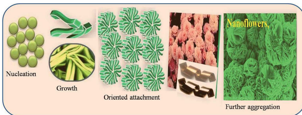
Scheme 1 Plausible mechanism for formation of 3D-nanoflower-like Cu foil coated with CuO (inset: photo image of undeposited and deposited CuO nanoflowers on flexible Cu foil by chemical bath deposition method).
