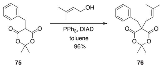
**Scheme 23** C-alkylation of C<sup>5</sup>-mono-substituted Meldrum's acids.
