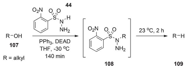
**Scheme 38** Deoxygenation of alcohols to alkanes using *o*-nitrobenzenesulfonylhydrazine **44**.
