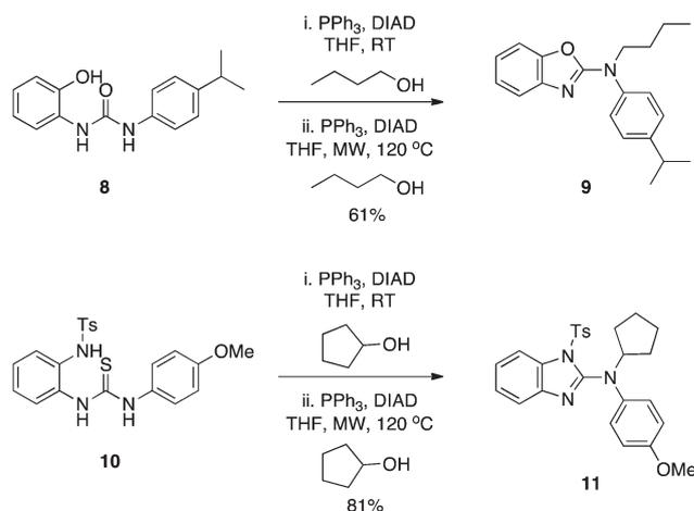
**Scheme 4** 2-Ureidophenols and tosyl-activated 2-thioureidoanilines undergo intramolecular Mitsunobu reactions to deliver *N*<sup>2</sup>-substituted benzoxazoles and benzimidazoles, respectively.
