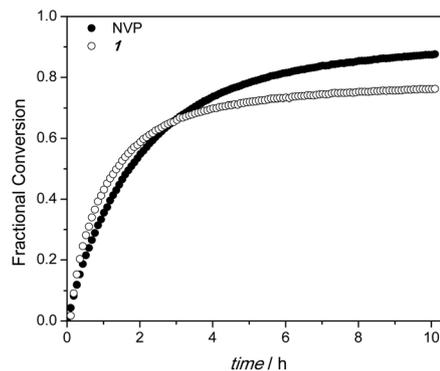
Fig. 2 Fractional conversion profiles for 1 and NVP monitored by *in situ* <sup>1</sup>H NMR during a polymerization carried out at 65 °C with [NVP]:[1]:[AIBN] = 5:1:0.1.
