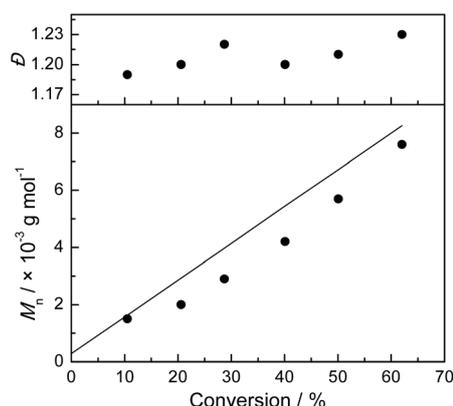
**Fig. 4** Evolution of  $M_n$  and  $\mathcal{D}$  as a function of conversion for NVP polymerization in semi-batch mode, using RAFT agent 1 (entry 3, Table 1).
