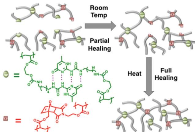
**Scheme 1** Synthesis and proposed healing mechanism of the PHEA-FMIDA-UPyA material. Initially the hydrogen bonded UPyA units join to partially heal the material. With thermal stimulus the covalently linked FMIDA units join across the interface.
