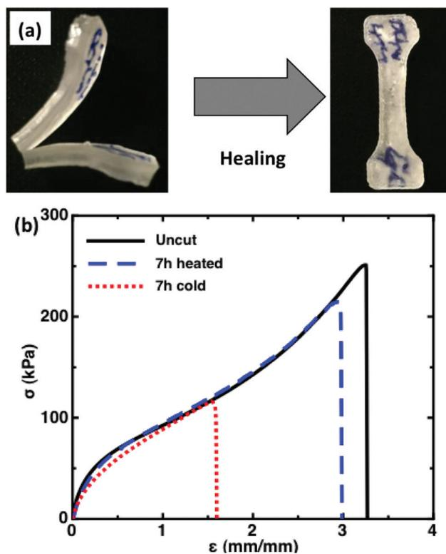
**Fig. 1** (a) Left shows the PHEA-FMIDA-UPyA material directly after being cut with a razor. Right shows the same material with the scratch being much less prominent after 7 h of room temperature healing. (b) Comparison between the uncut and the PHEA-FMIDA-UPyA materials that were cut and healed under cold conditions for 7 h (room temperature) and cut and heated at  $90\text{ }^\circ\text{C}$  for 7 h.
